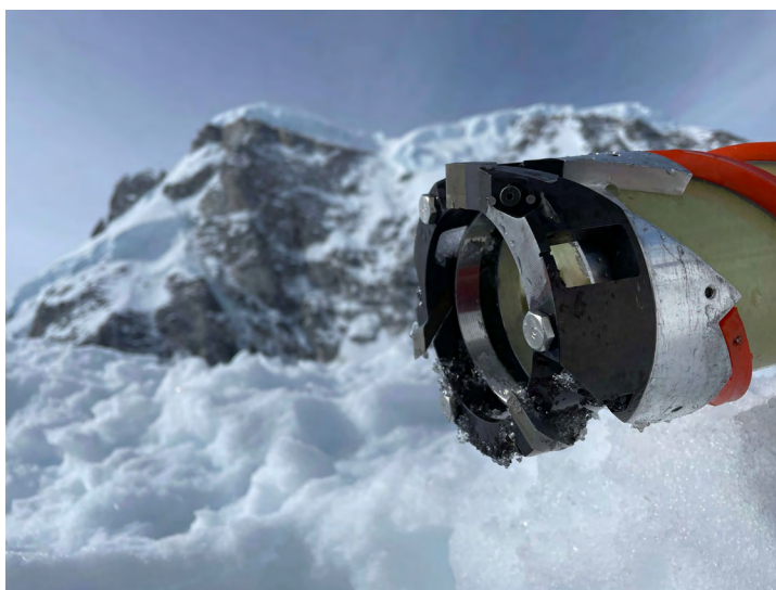
(Top) Julia Andreasen logs a core drilled with the IDDO Hand Auger at Combatant Col, British Columbia, Canada. Credit: Peter Neff. (Bottom) A close-up view of the IDDO Hand Auger cutter head. Credit: Peter Neff.
