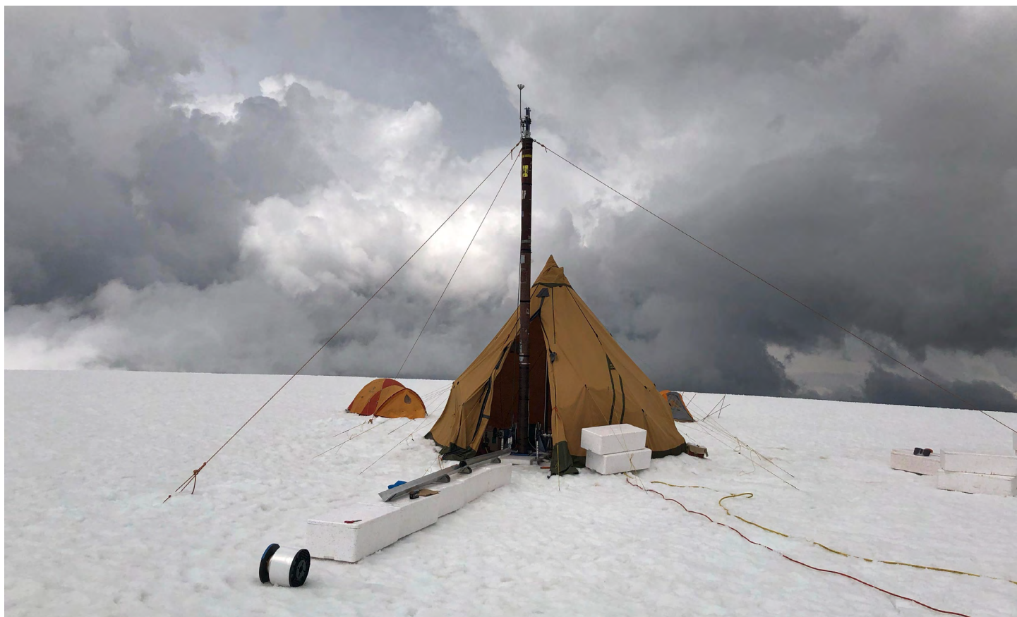
The Electrothermal (aka Thermal) Drill on the Quelccaya Ice Cap, Peru. The Electrothermal Drill was chosen because it works well in locations where the ice is close to its pressure melting point. In such situations, the more common electromechanical drills are at risk of getting stuck from melting and refreezing of the surrounding ice. The Electrothermal Drill uses a ring-shaped heating element in the coring head to melt an annulus around the ice to be cored, rather than shaving it away with cutters like electromechanical drills. Credit: Elliot Moravec.
