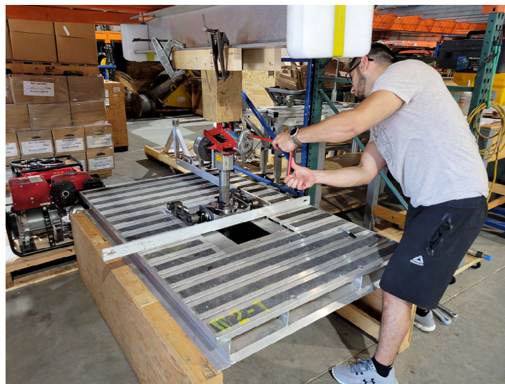
(Top, Right) A Stampfli Drill core barrel is adapted for use with the Chipmunk Drill and tested in a chest freezer. Credit: Jay Johnson; (Bottom, Left) Electrical engineers conduct comprehensive testing on Foro 3000 Drill electronics. Credit: Jay Johnson; (Bottom, Right) The new Winkie Drill slip-style foot clamp is load tested. Credit: Jay Johnson.
