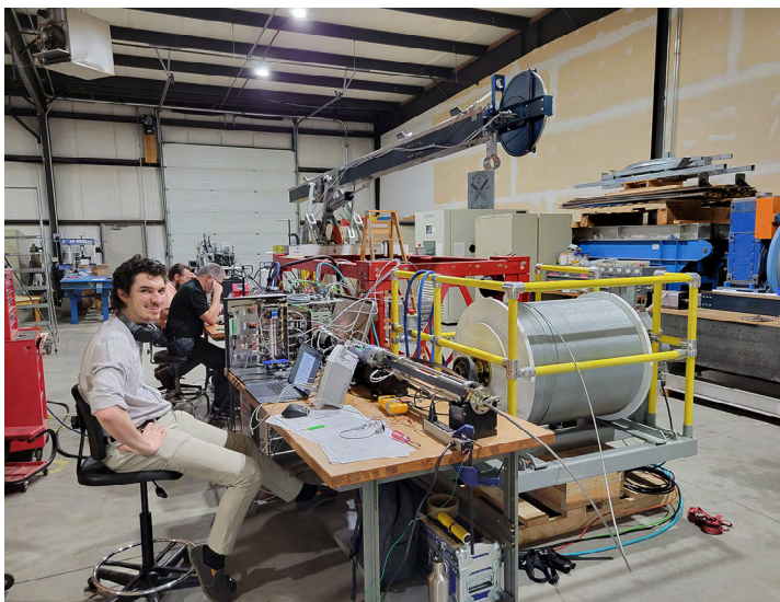
(Top, Right) A Stampfli Drill core barrel is adapted for use with the Chipmunk Drill and tested in a chest freezer. Credit: Jay Johnson; (Bottom, Left) Electrical engineers conduct comprehensive testing on Foro 3000 Drill electronics. Credit: Jay Johnson; (Bottom, Right) The new Winkie Drill slip-style foot clamp is load tested. Credit: Jay Johnson.
