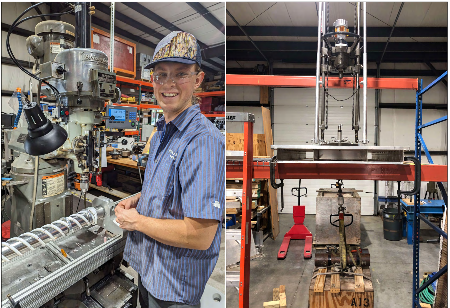
(Left) Elliot Moravec installs flights on the 700 Drill core barrels. Assembly of the sonde is nearly complete, from the anti-torque section down to the cutter head. Credit: Jess Ackerman. (Right) Winkie Drill test setup at the IDP facility in Madison, WI. Credit: Elliot Moravec.
