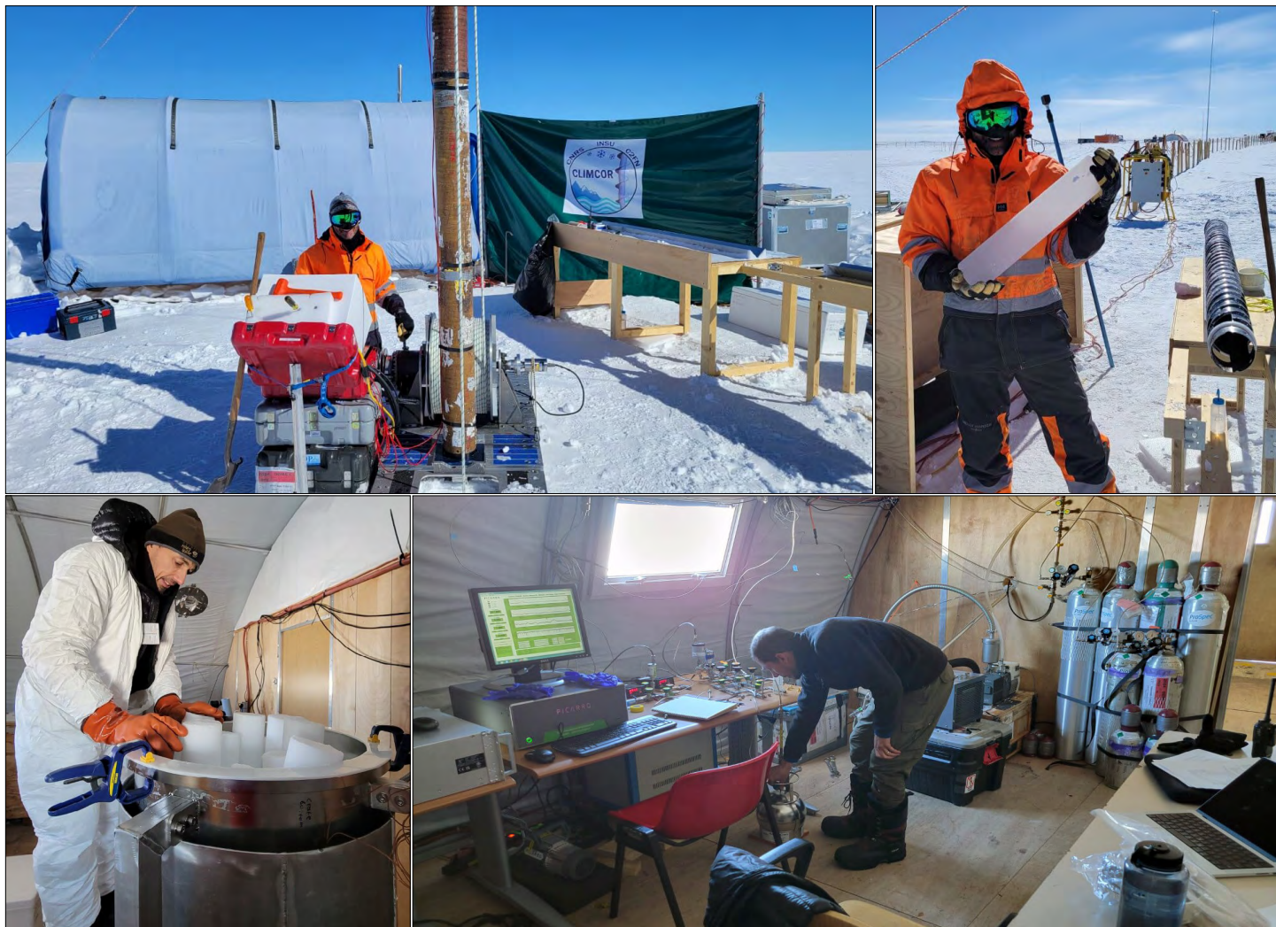
(Top, Left) Jay Johnson operates the 4-Inch Drill at Dome C, Antarctica. Credit: Alexander Ihle. (Top, Right) Jay Johnson holds the last core segment from the second borehole drilled with the 4-Inch Drill. Credit: Alexander Ihle. (Bottom, Left) Vas Petrenko loads the onsite melter to extract the air from the ice cores for analyses of carbon monoxide and methane isotopes. Credit: Jay Johnson. (Bottom, Right) Vas Petrenko fills a sample canister with the extracted air. Credit: Jay Johnson.
