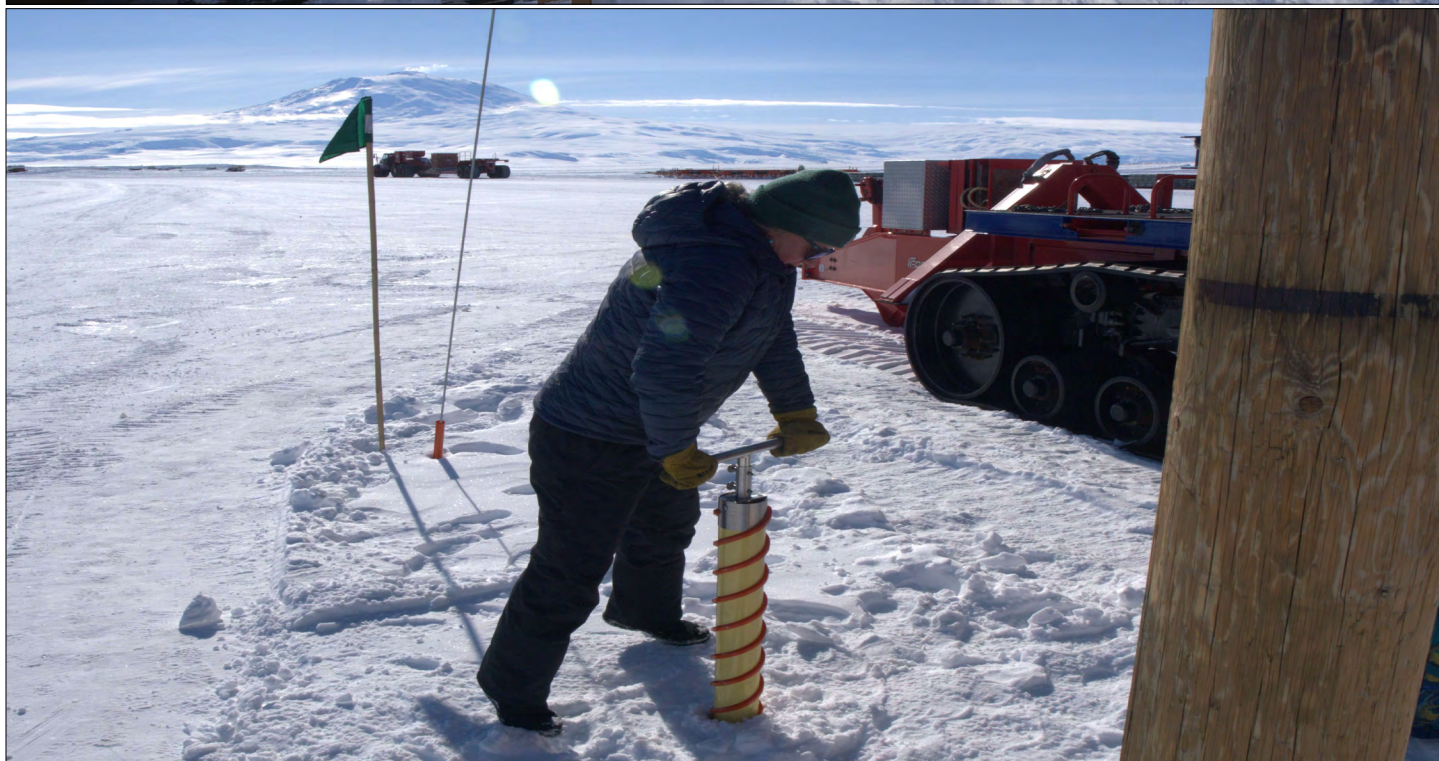
(Top) Julie Webber (McMurdo Station Crary Lab, left), Parker Steen (Massachusetts Institute of Technology, middle) and Stine Ornes (USAP Field Safety, right) use a Kovacs Mark II hand auger on the Ross Ice Shelf, Antarctica, to measure the density of the Ross Ice Shelf firn. Credit: Bryan Minnear, Lead Pilot, Pathfinder Systems. (Bottom) Julie Webber (McMurdo Station Crary Lab) tests the Kovacs Mark II hand auger on the McMurdo Ice Shelf. Credit: Parker Steen (Massachusetts Institute of Technology).
