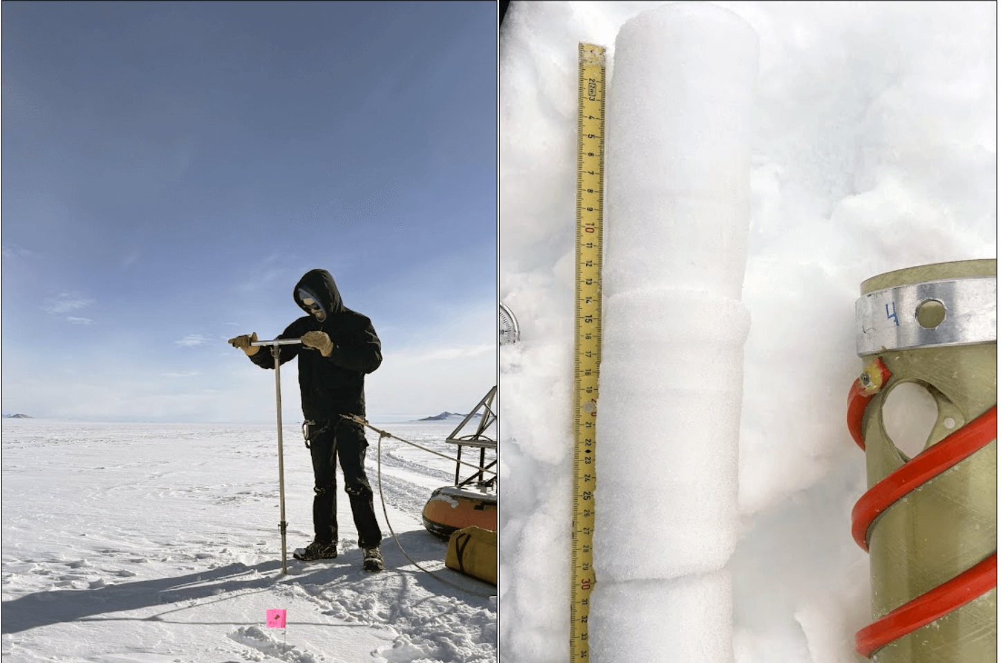
(Left) Derek Pickell (Dartmouth College) uses the IDP hand auger to examine crevasse bridge properties at the base of the Leverett Glacier, Antarctica. The pink flag denotes the center of the crevasse bridge as identified by ground penetrating radar. Credit: Zoe Courville. (Right) One of the shallow cores collected from a crevasse bridge at the base of the Leverett Glacier. The team drilled several cores on and off the crevasse bridges they found and used the cores to study stratigraphy, grain sizes, and density. Credit: Zoe Courville.
