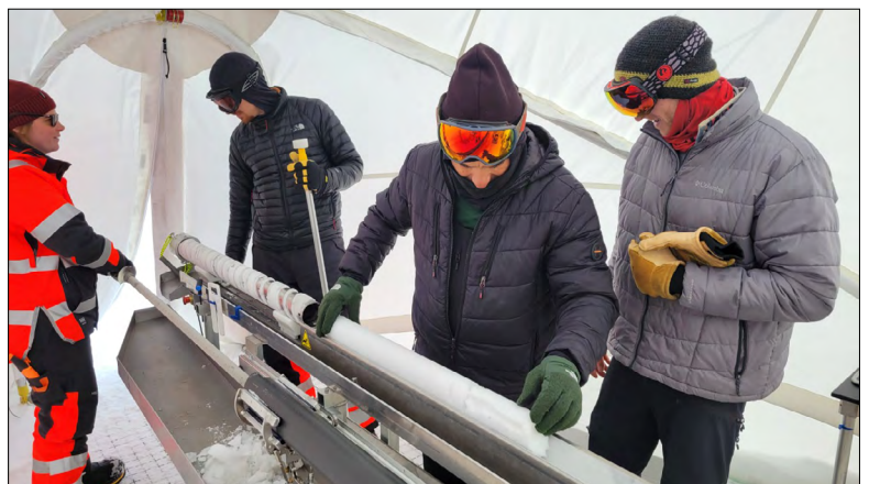
At Summit, Greenland, Murat Aydin measures the length of the first core drilled with the 700 Drill. Credit: Jay Johnson.
