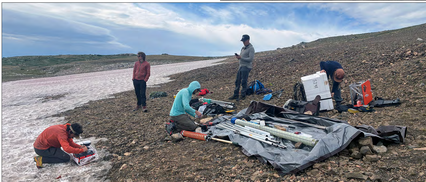
(Top) The science team led by Dr. Nathan Chellman (DRI) operate the IDDO Hand Auger on the Chugach National Forest Ice Patch in Alaska. Credit: Tanner Kuhl. (Bottom) The science team prepares equipment to begin fieldwork on the Tolman Ice Patch, Wyoming. The IDDO Hand Auger is the barrel with the orange flights. The Prairie Dog Drill is the greenish-looking barrel resting on top of the grey tarp. Credit: Elliot Moravec.
