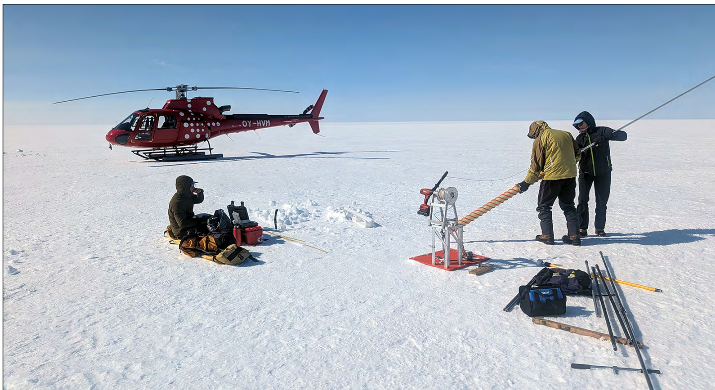
Dr. Joel Harper (University of Montana) and team operate the IDDO Hand Auger and Sidewinder to collect cores in Greenland during the 2026 field season. The field site was accessed via an Airbus H125 (AS350) helicopter. Credit: Joel Harper.
