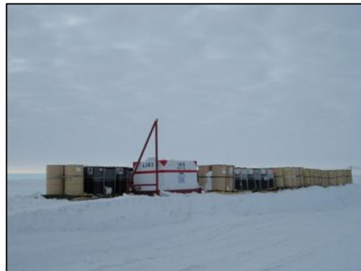
Drill fluid drums and a sled mounted storage tank used at WAIS Divide
