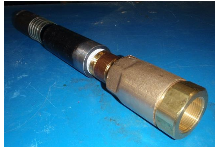
Fluid Bailer Check Valve from ASIG Drill
