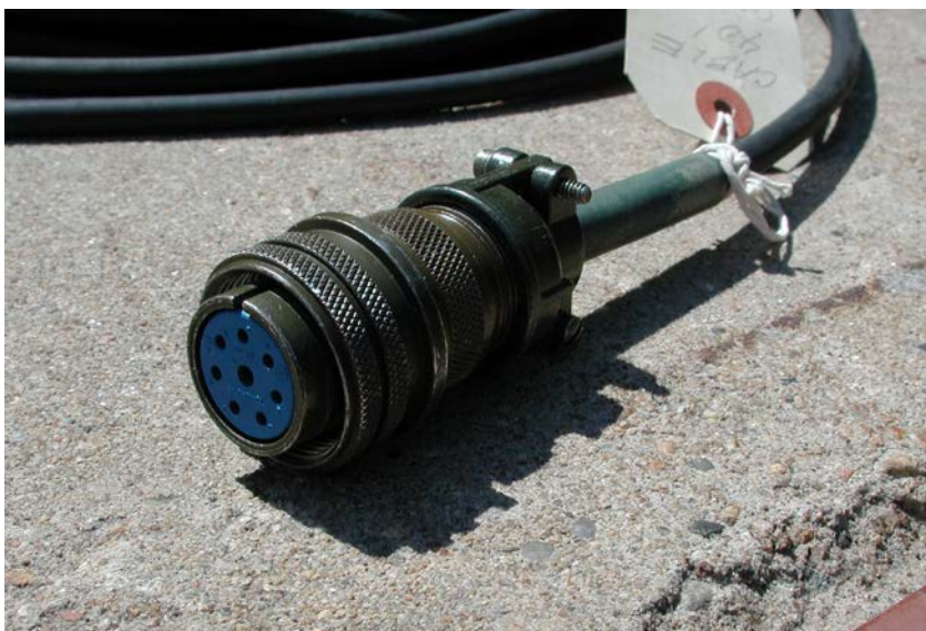
Figure 7. Example of cable needed to connect the logging instruments to the slip-ring connector.
