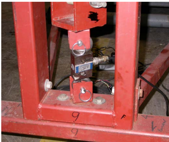
Figure 9. Load cell used for measuring cable tension.
