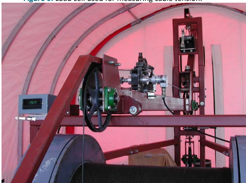
Figure 10. Digital readout showing cable tension is on the left.
