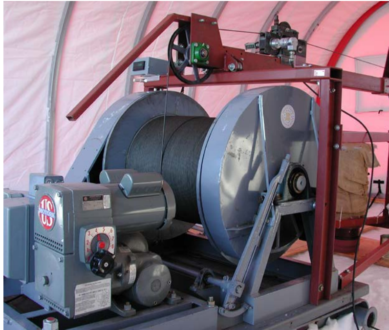
Figure 1. Photo showing the drum, hand brake, and motor assembly. Logging speed is controlled by the dial on the varidrive unit.
