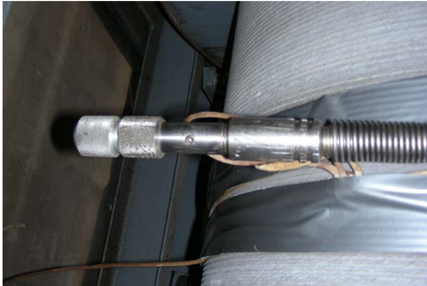
Figure 5. Cable head with protective cap in place. Before every deep logging run, arctic grease (or equivalent) should be injected into the cable head by replacing the set screw in the middle of the narrow section with a zerk fitting. A special tool is needed to remove the spring (right side) from the cable head.
