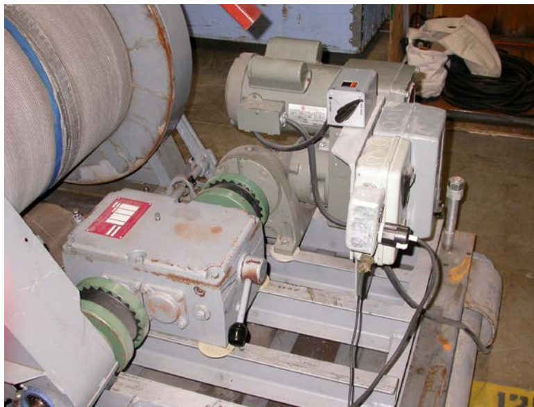
Figure 2. Power created by the motor passes through a sure-flex coupling, the transmission, another sure-flex coupling, and into the drive sprocket (blue housing, lower left).
