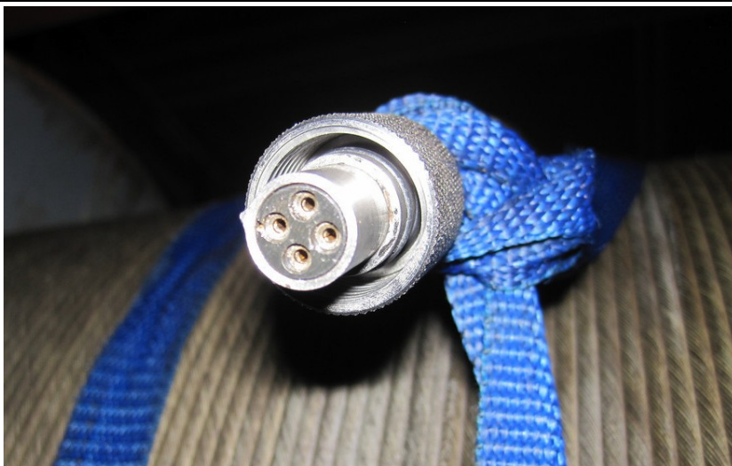
Figure 6. End view of the cable head. O-rings are just barely visible under threaded shell. Logging tools need to be compatible with this cable head.
