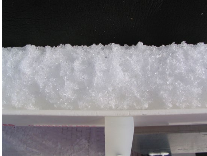
Figure 13-2: Large crystals of the firn ice core.
