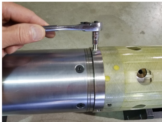
Figure 9-16: Motor section to outer barrel connection.
