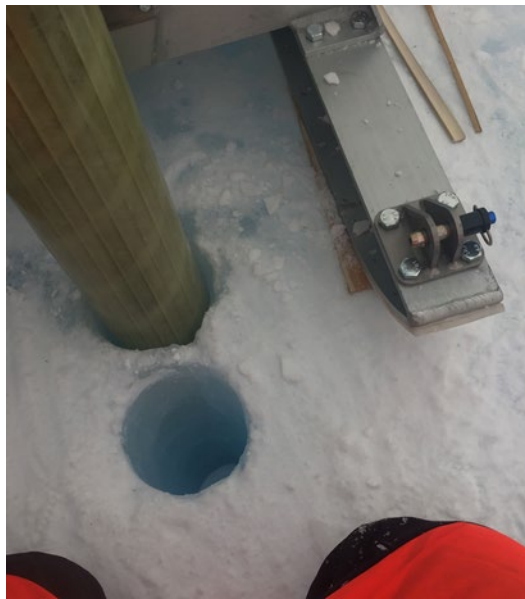
Figure 12-5: Shallow hole drilled in front of the main borehole to facilitate barrel disassembly.
