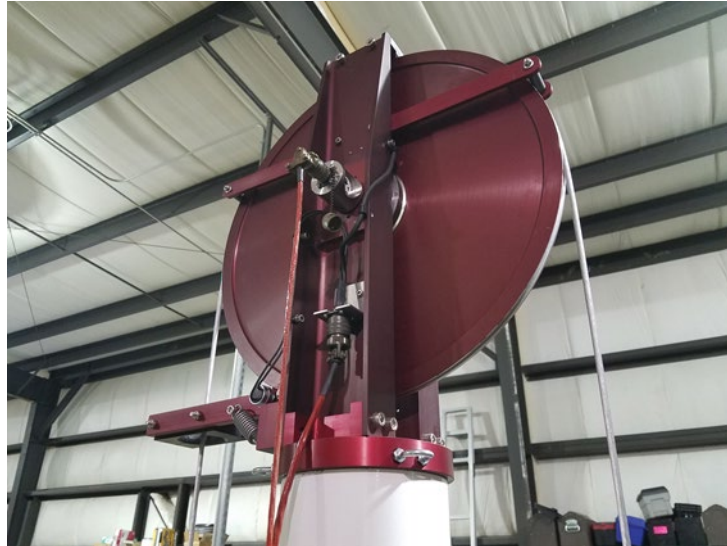
Figure 9-8: Crown sheave assembled to top tower section.
