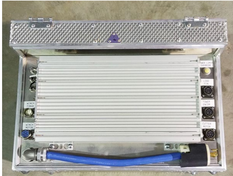
Figure 9-21: Control box cable connections.
