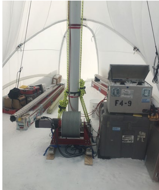
Figure 9-23: Control box setup with the drill system and core processing station at left.
