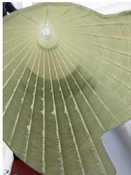
Figure 13-6: Iced-up grooves in outer barrel.
