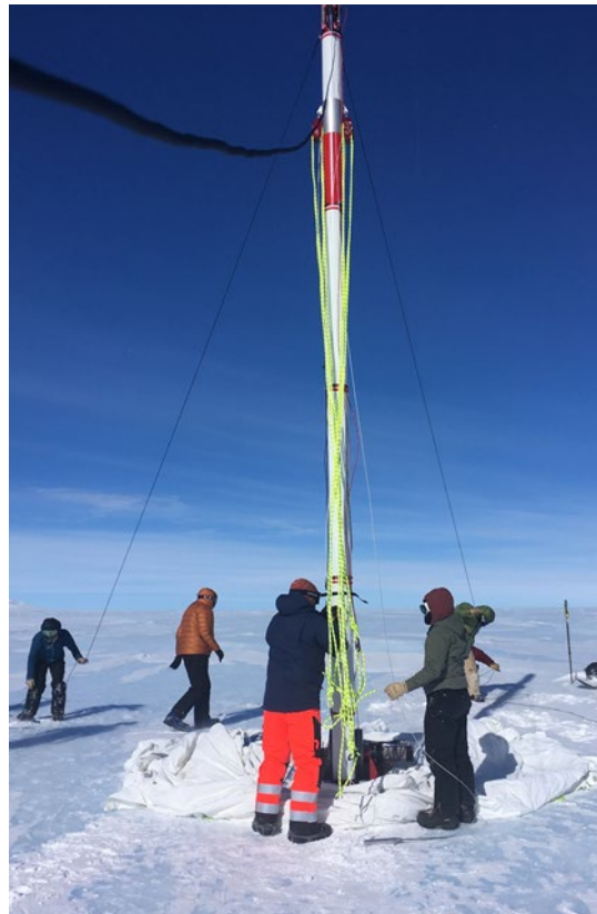
Figure 12-1: Raising the drill tower with drill tent body and rigging.
