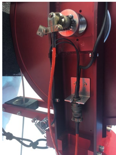
Figure 9-22: Crown sheave assembly showing load pin and cable, encoder cable, and hard limit switch.
