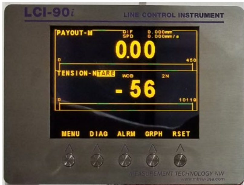
Figure 13-1: LCI-90i screen on the faceplate of the Foro Drill Control.
