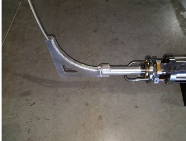
Figure 12-3: Cable guide used while raising drill string onto tower.
