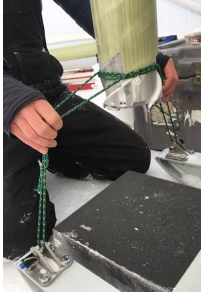
Figure 13-7: Winching apart stuck barrels with thick foam covering borehole to protect cutters.
