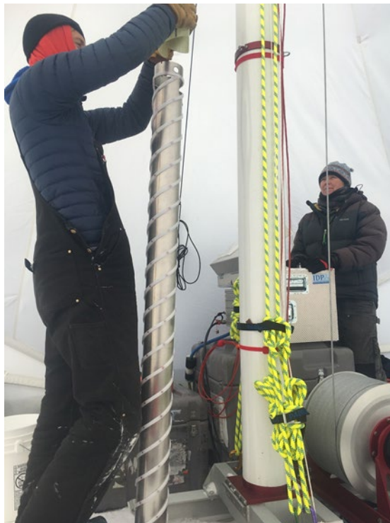
Figure 12-4: Lowering drill string over core barrel.
