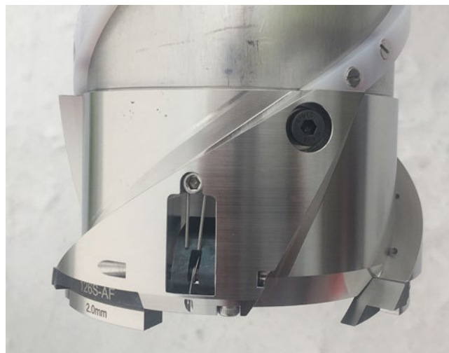
Figure 9-19: Cutter head with long core dogs, step cutters, and 2.0 mm shoes.
