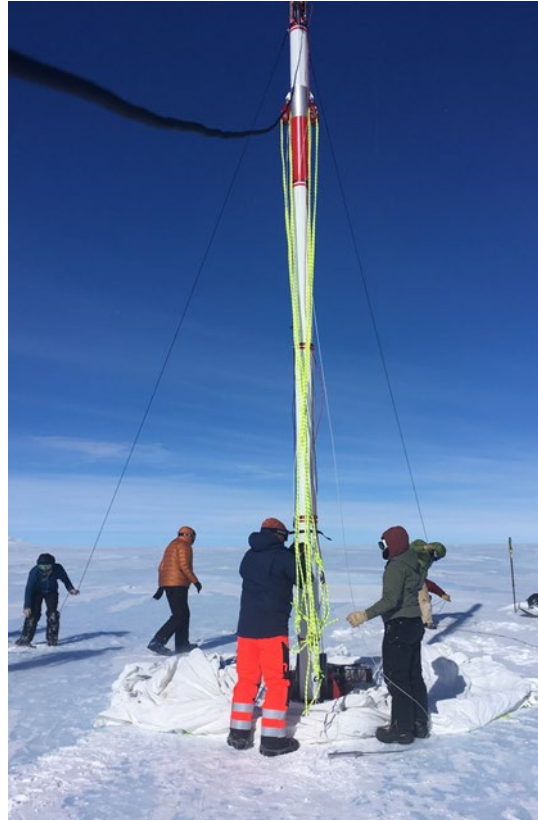
Figure 12-1: Raising the drill tower with drill tent body and rigging.
