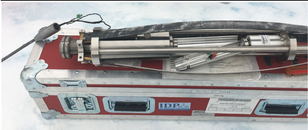
Figure 9-13: Attaching the drill cable termination to the AT section.
