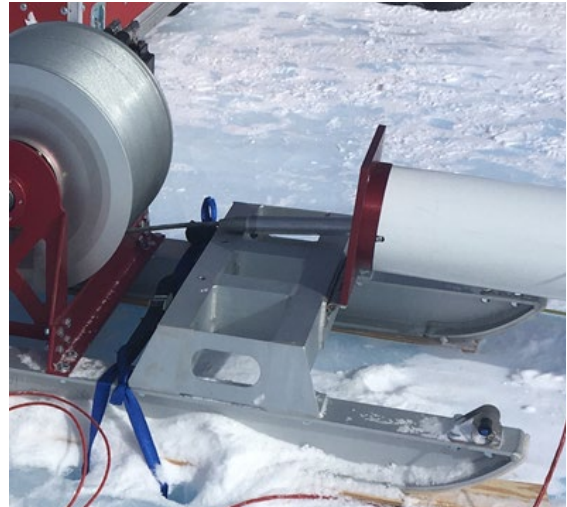
Figure 9-4: Tilted tower base showing keyed connection to bottom tower section.
