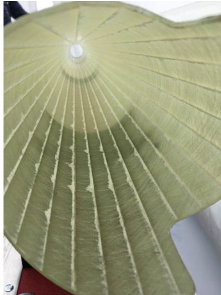
Figure 13-6: Iced-up grooves in outer barrel.
