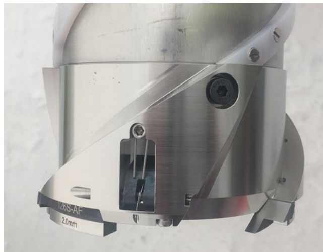
Figure 9-16: Cutter head with long core dogs, step cutters, and 2.0 mm shoes.
