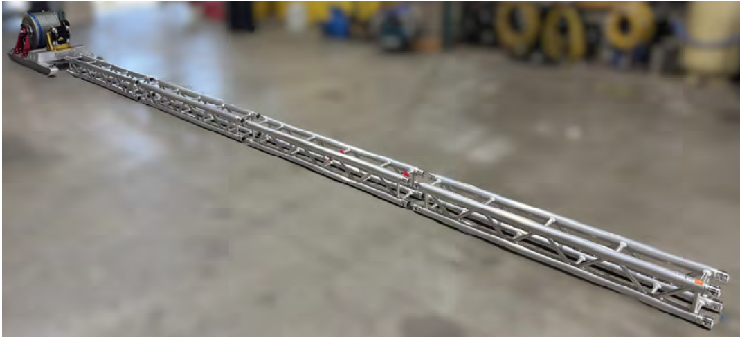
Figure 9-2: Truss sections prepared for assembly.
