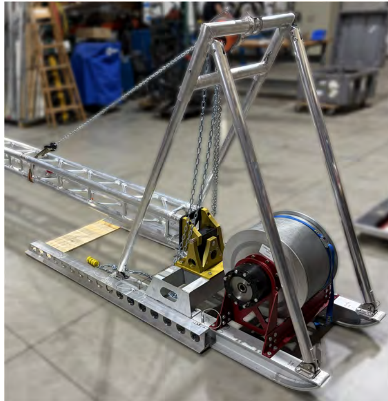
Figure 12-1: Tower lifting frame assembly attached to the winch sled.
