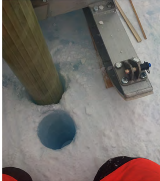
Figure 12-8: Shallow hole drilled in front of the main borehole to facilitate barrel disassembly.
