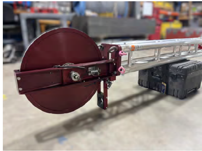
Figure 9-5: Crown sheave assembled to top tower section.
