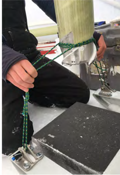
Figure 13-7: Winching apart stuck barrels with thick foam covering borehole to protect cutters.
