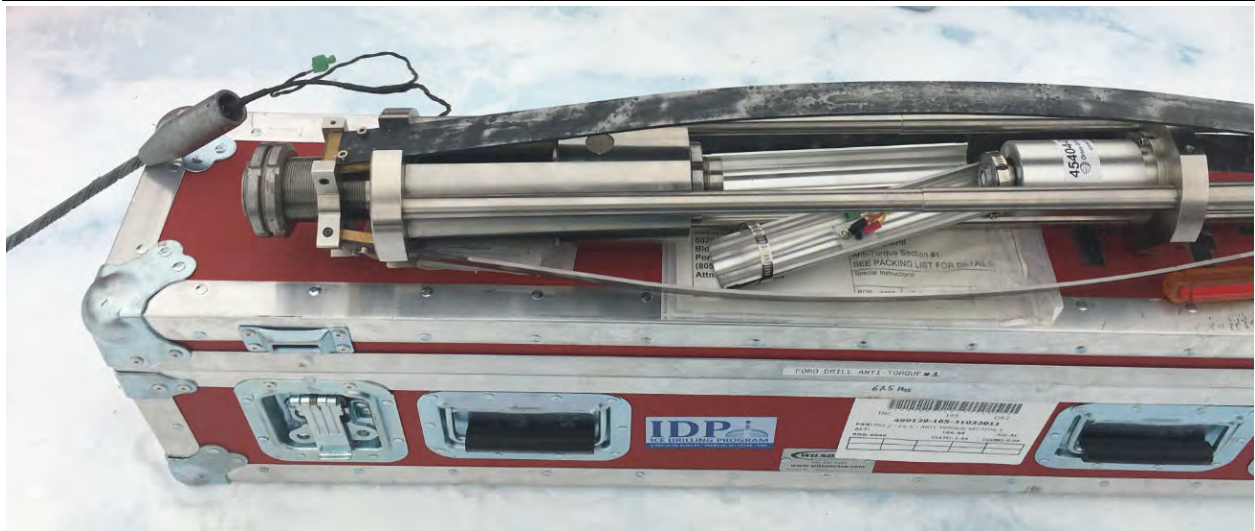
Figure 9-10: Attaching the drill cable termination to the AT section.
