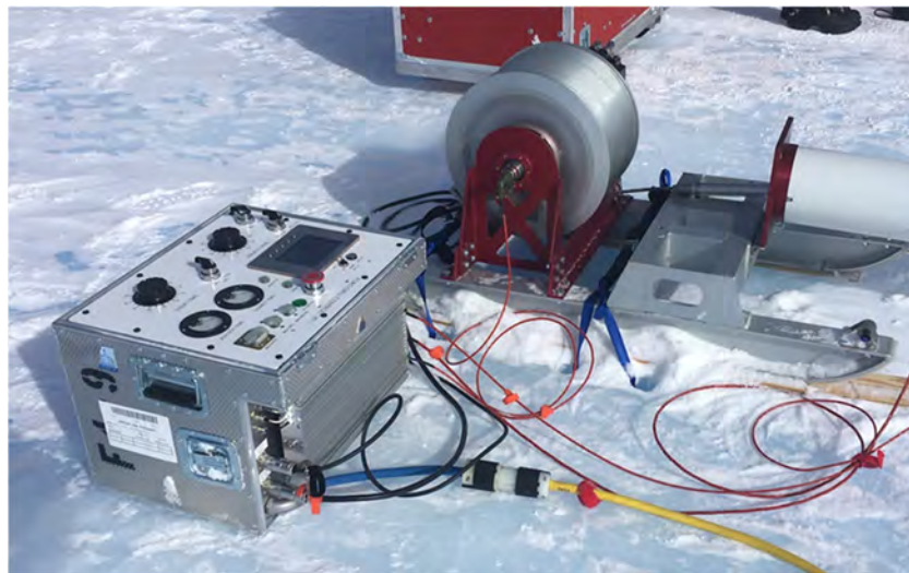
Figure 9-8: Control box and winch, showing the electrical slip-ring connection.
