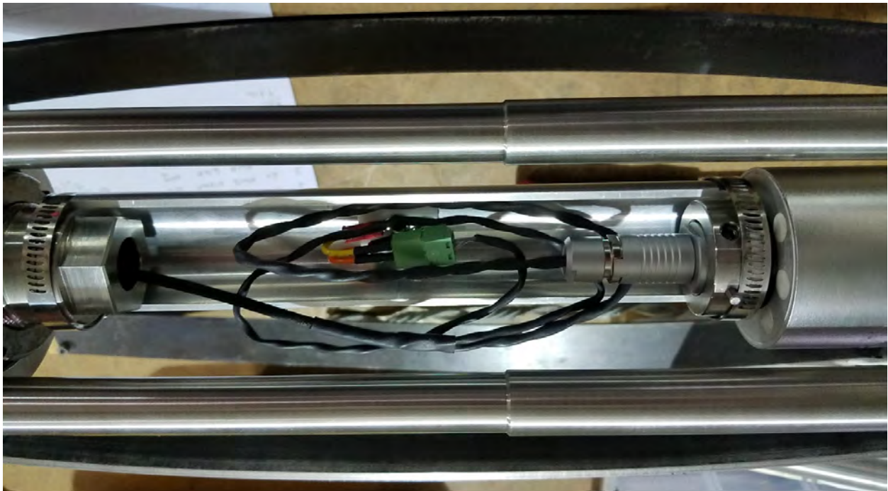
Figure 9-12: The cable assembly inside the torsion cover clamshell.
