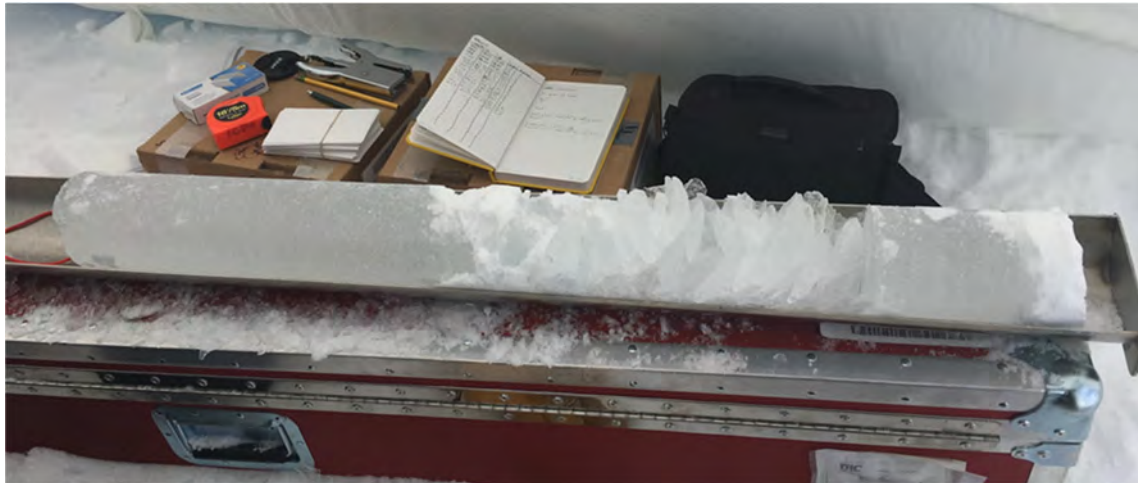
Figure 13-3: Rubble section in middle of core corresponding to low tension while coring.
