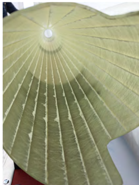
Figure 13-6: Iced-up grooves in outer barrel.
