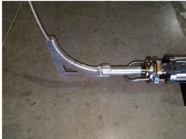
Figure 12-6: Cable guide used while raising drill string onto tower.
