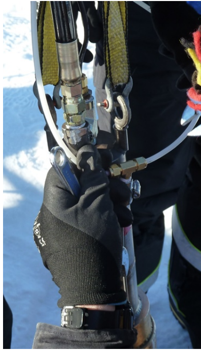
Figure 3: Installing dual inflation lines at the tee above the packer
