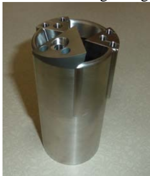
Figure 6: ASIG Ice Cutter Head Custom ice drilling head shown with one of three cutters in position
