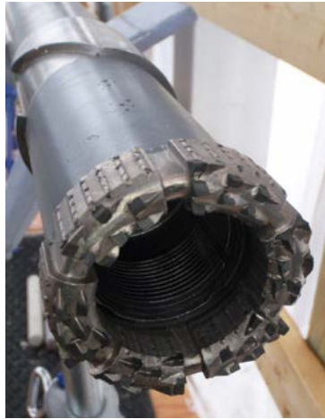
Figure 8: GeoSet Diamond Bit used for Mixed Ice/Rock Coring
