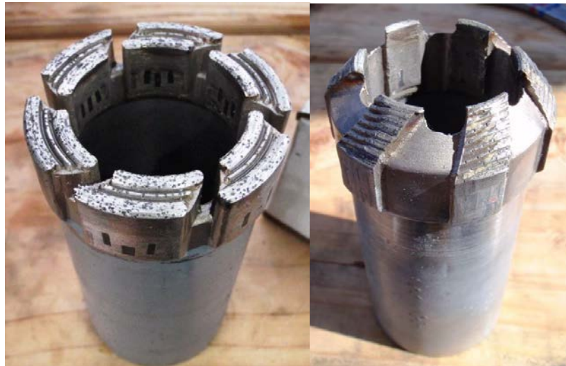
Figure 7: Coring Bits - At left, Diamond-impregnated coring bit; at right, worn QD Tech Hybrid coring bit for mixed ice/rock coring.
