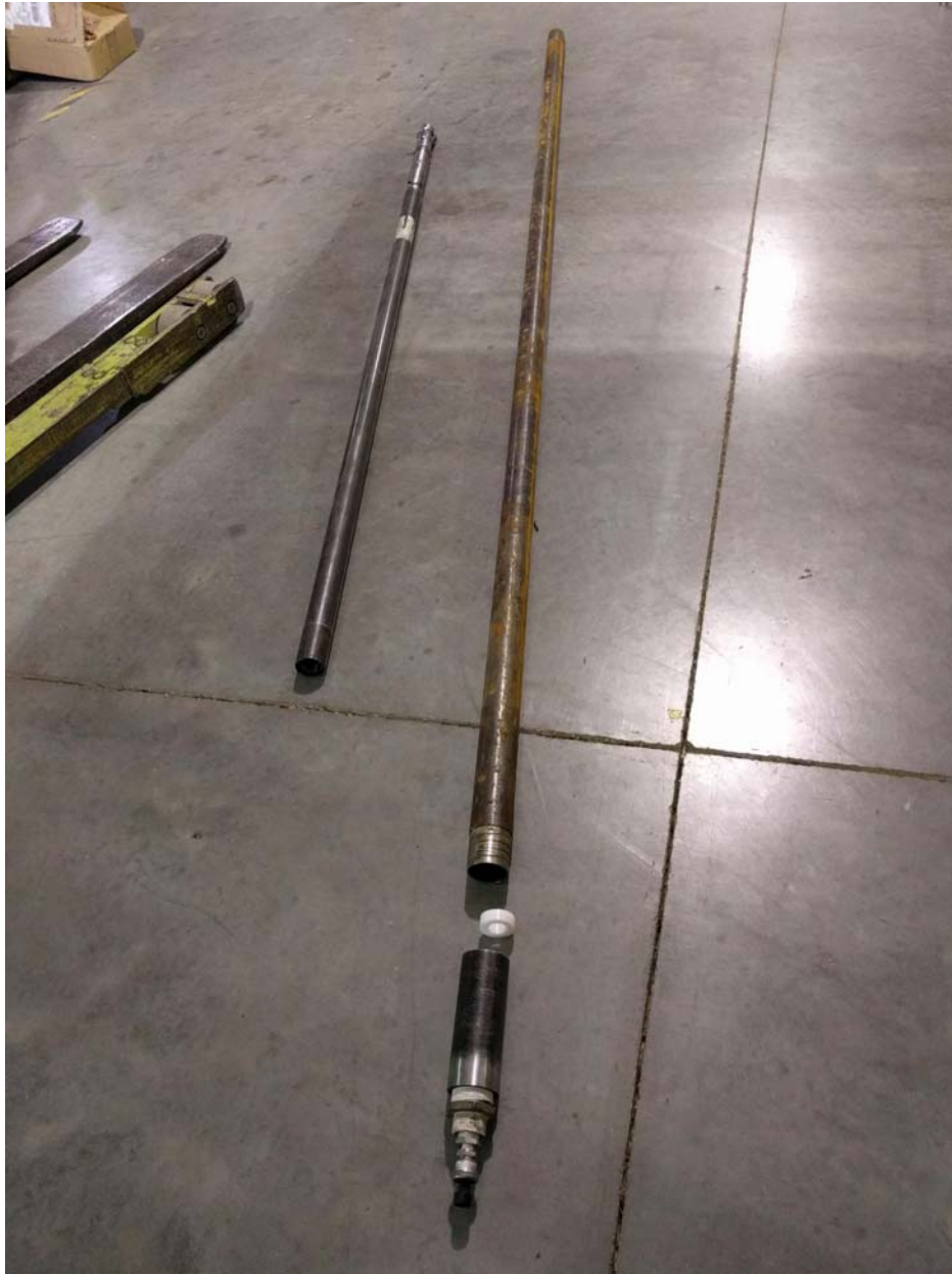
Figure 2: Core Barrel Assembly (left), Drill Rod Assembly (right) including drill rod, plastic spacer ring, sub-adapter and pressure transducer. The plastic spacer was included to prevent the core tube from being damaged on impact with the sub-adapter.
