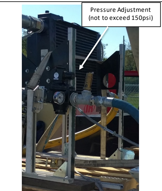
Fig. 4: Regulator and Safety Relief Valve
