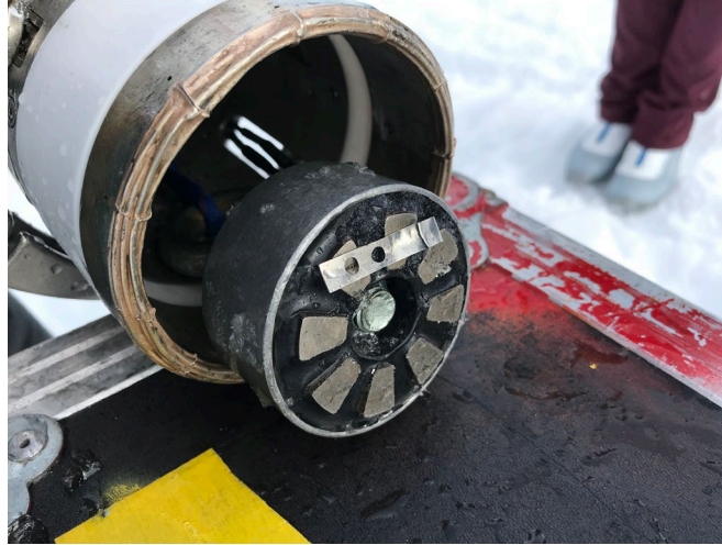
Figure 1. A magnet can be used to retrieve steel debris downhole.
