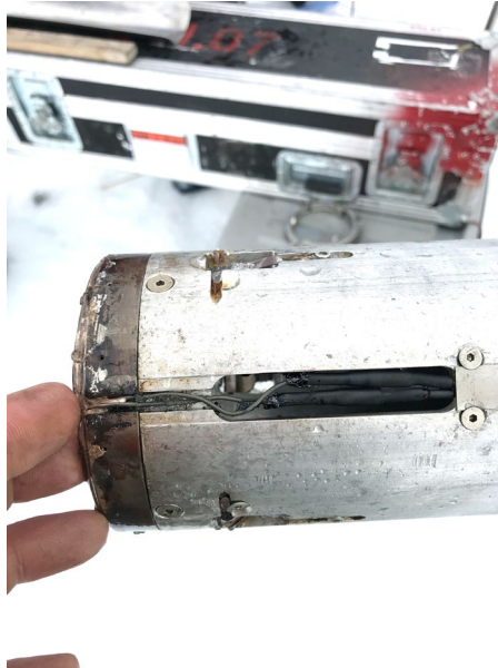
Figure 7. Connection between heat ring and drill cable.
