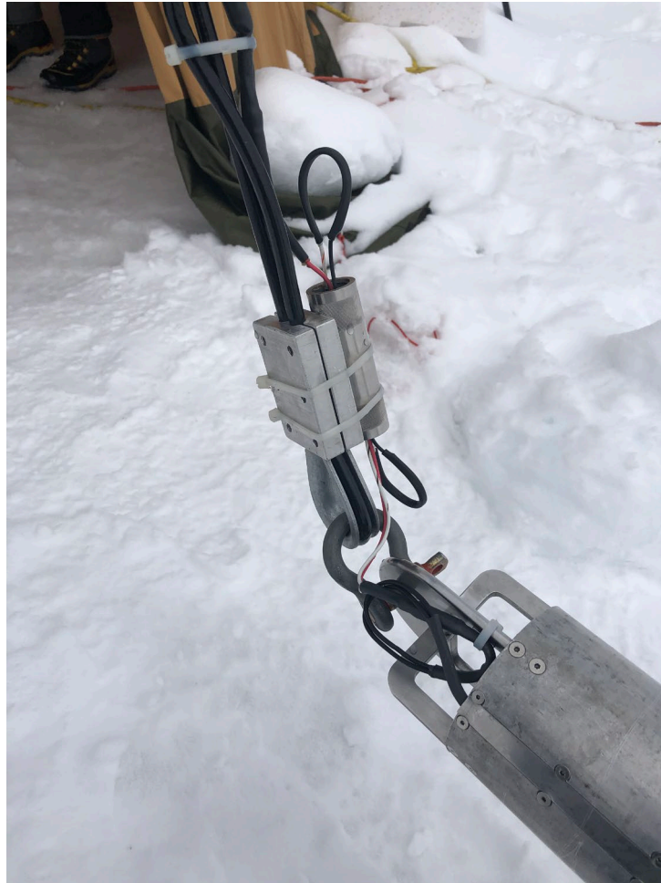
Figure 3. Thermal drill mechanical and electrical connections.
