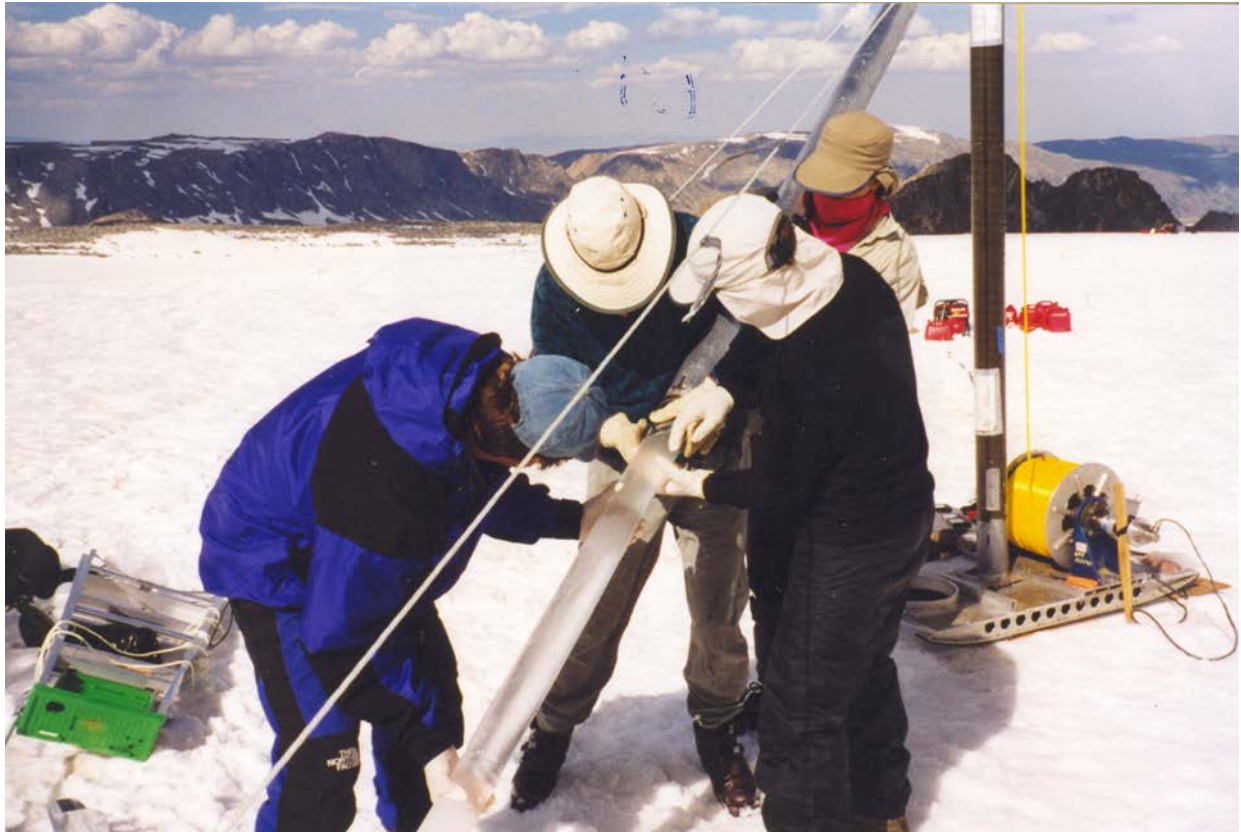
Picture 2: Extracting the core from the Thermal Drill sonde. This was the second drilling of the Fremont Glacier in the Wind River Range of Wyoming. Notice the yellow cable. It is co-axial with Kevlar reinforcement. The cable length is 200 meters and is spooled onto the 100-meter winch sled designed for use with the 4-Inch Drill. Here, the tower is of smaller diameter fiberglass/epoxy tubing that serves also as a shipping tube for Thermal Drill. The tower base that hinges on the sled was modified as was the sheave. This was a weight savings of 150 pounds over the 200-meter winch sled.
