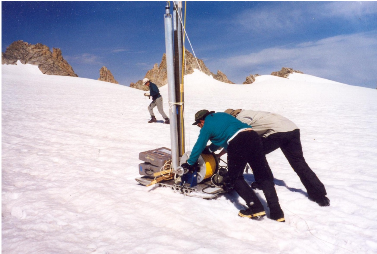
Picture 5: Moving the drilling sled to a new location. The Thermal Drill is tied to the tower. Moving equipment over the soft snow requires a lot of effort.
