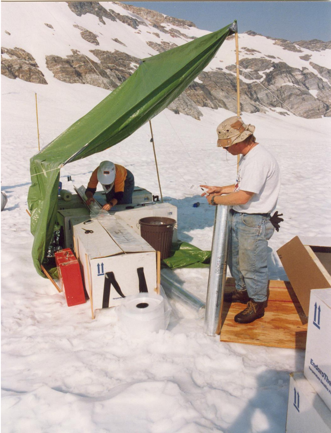
Picture 6: Core processing in the shade on the South Cascade Glacier in Washington State near the Canada border. Makeshift shade is very important because the solar input can be intense at altitude.
