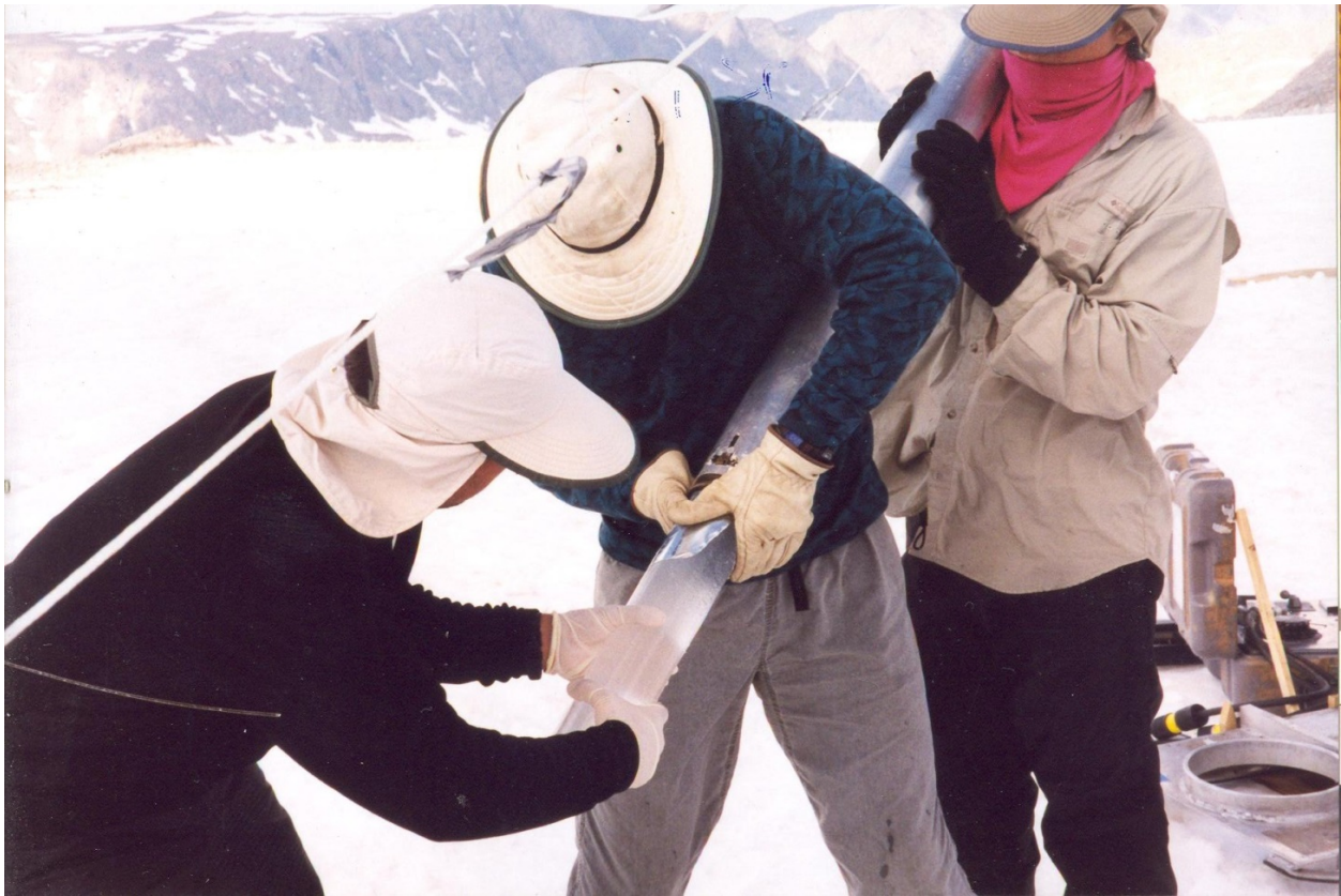
Picture 4: Using the stovepipe to hold back the core dogs, the scientists allow the core to slide out the end. The stovepipe is inserted by placing it around one's hand as the hand pushes the core up, relieving the pressure on the dogs. Then, it is slid along the inner surface of the drill barrel alongside the core until the core dogs are pressed back.
