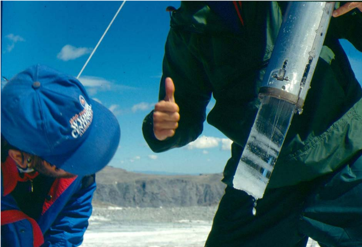
Picture 1: The first drilling project with the Thermal Drill. The project was conducted on Fremont Glacier in the Wind River Range of Wyoming where a core of 150+ meters was drilled. The core dog setup worked almost without flaw. One can see the heat ring mounted to the bottom of the core barrel as well as the groove cover that runs along the side of the barrel. Each heat ring has a 2-wire 'tail' that is over two meters length. The cutout, seen between the heat ring and the groove accommodates the joints of the heating element to the wire tail.
