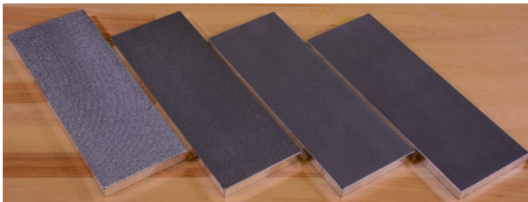
Figure 41. Atoma Diamond Plates. From left to right, 140-grit, 400-grit, 600-grit, 1200-grit.
