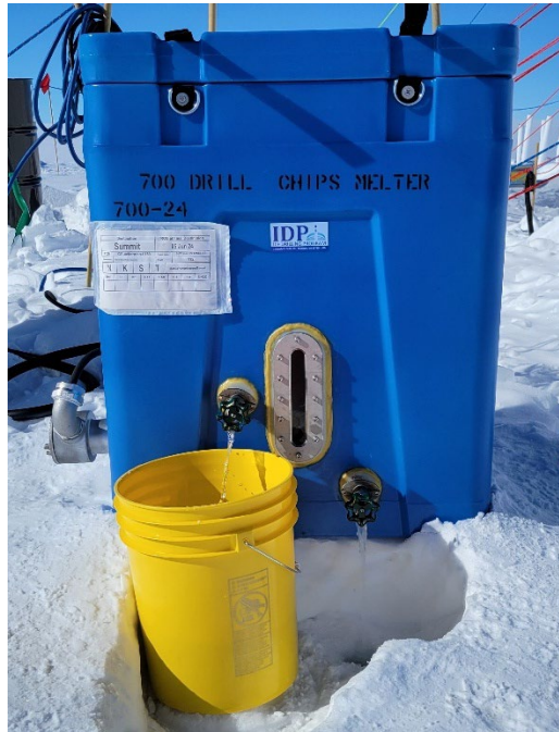
Figure 14. The chip melter has an upper and lower valve and sight glass on the front. When the transition between water and drilling fluid is visible between the valves in the sight glass, water can be drained from the lower valve and drilling fluid from the upper valve.
