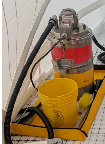
Figure 16. Industrial vacuum for picking up drilling fluid and ice cuttings.
