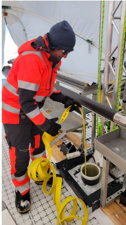
Figure 18. Yellow layflat fire hose is used to add drilling fluid to the borehole below the firn-ice transition.
