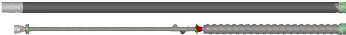
Figure 8. Barrel Set components include the outer tube, hollow shaft assembly, core barrel, and cutter head assembly.
