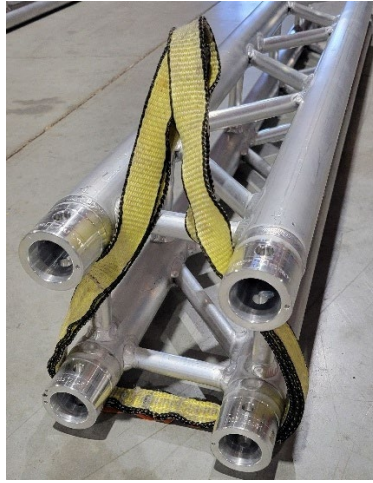
Figure 24. Tower lifting strap placement.
