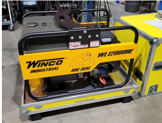
Figure 1. Image of one generator on its ATA case base.
