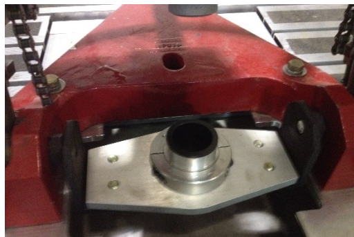
Fig. 3. Unipress base and rod guide assembly. NOTE: 3/4-10 hex bolts have been extended and jam nut must be used to prevent loosening from vibration.
