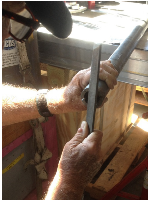
Fig. 14. A bastard file is used to dress the bit; disrupt the surface of the bit to promote matrix wear and expose new diamonds at the beginning of each run.
