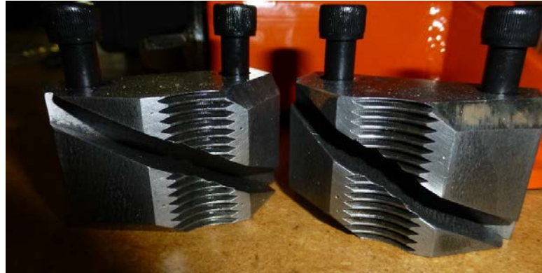
Fig. 19. Specialized Kwik Klamp jaws for use with Kovacs Enterprises augers.
