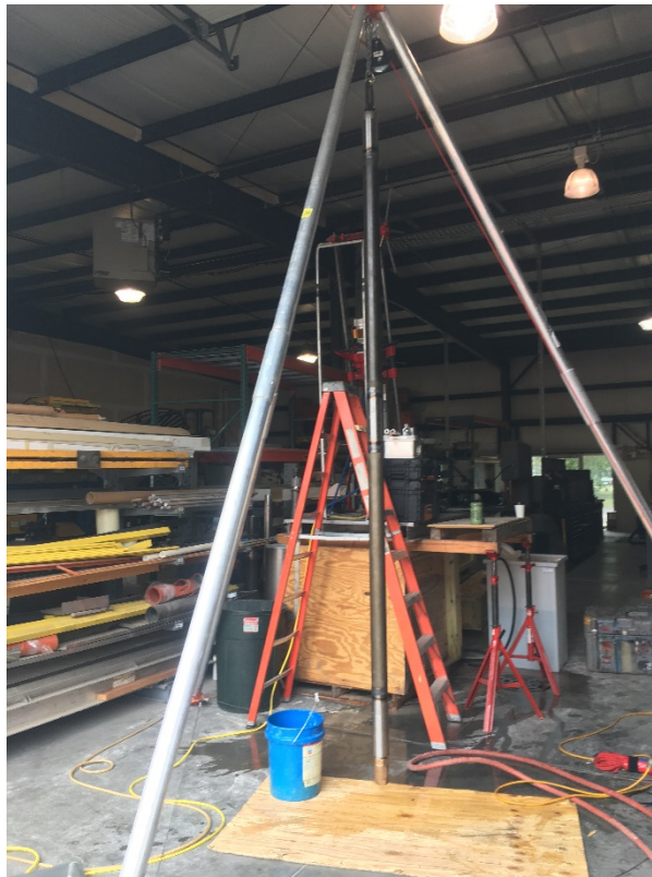
Fig. 9. Tripod with suspended drill rod and bailer sub adapter.
