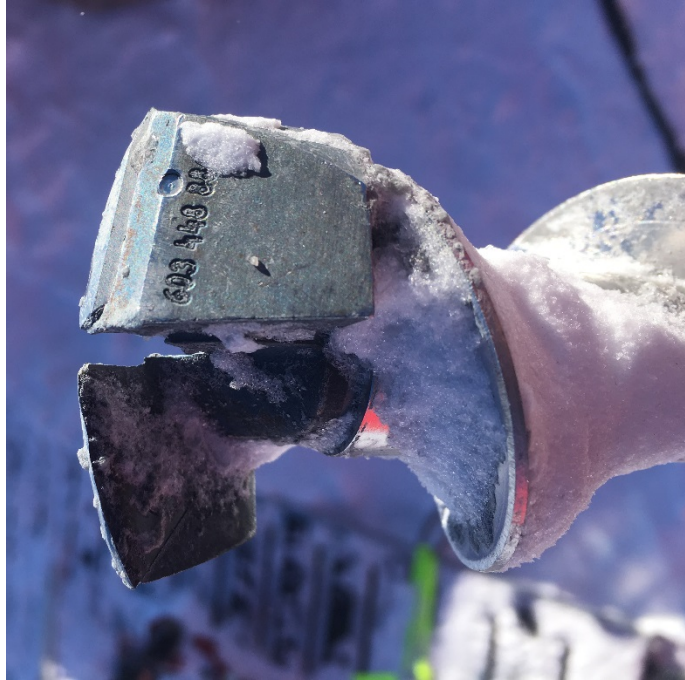
Fig. 18. Auger cutter head. Note the outside edge of the cutters are dulled from contact with bedrock.
