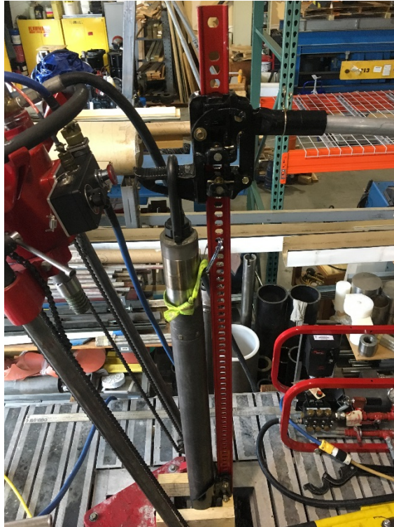
Fig. 15. Hi-lift jack positioned to break a rock core with the 86T2 coring barrel assembly.
