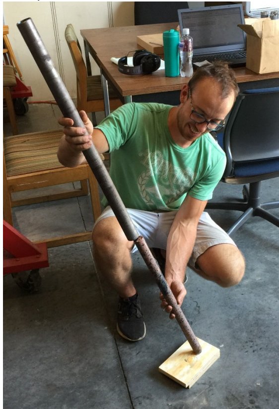
Figure 23: Removing rock core from AW34 core barrel.
