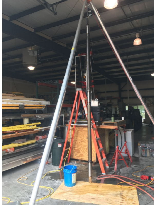
Figure 9: Tripod with suspended fluid bailer.
