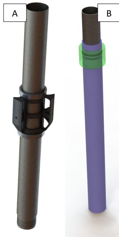
Figure: 10. (A) Centralizer installed with aluminum collars for free rotation. (B) Freeze-in casing shoe with polished steel casing nose piece.
