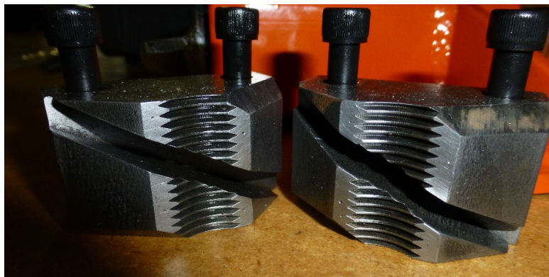
Figure 26: Specialized Kwik Klamp jaws for use with Kovacs Enterprises augers.
