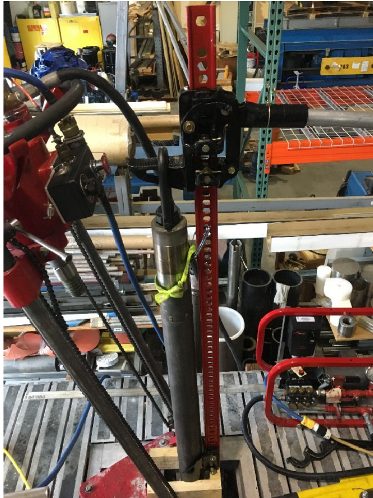
Figure 22: Hi-lift jack positioned to break a rock core with the 86T2 coring barrel assembly.
