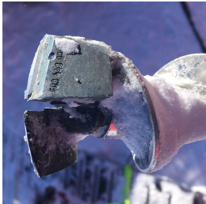
Figure 25: Kovacs auger cutter head. Note the outside edge of the cutters are dulled from contact with bedrock.
