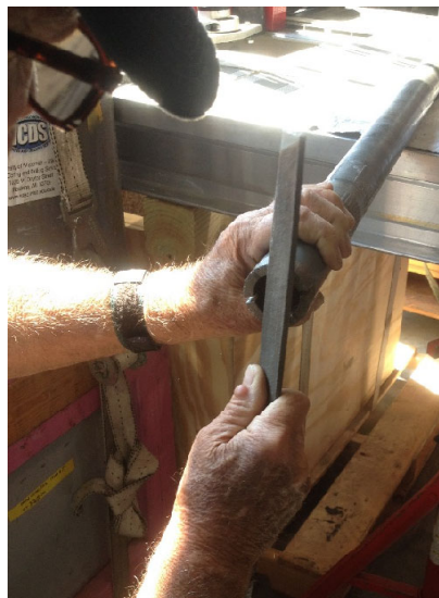
Figure 19: A bastard file is used to dress the bit; disrupt the surface of the bit to promote matrix wear and expose new diamonds at the beginning of each run.
