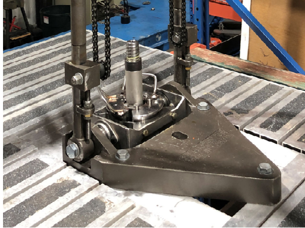
Figure 6: The slip foot clamp assembly. Note different diameter jaws exist for casing and drill rod.
