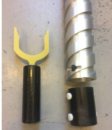
Figure 9: Barrel clutch adapter and separator tool
