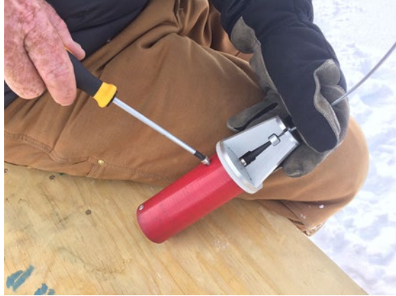
Figure 5: Removing the cable head cover
