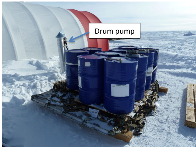
Figure 26. Pallet of drilling fluid outside the drill tent
