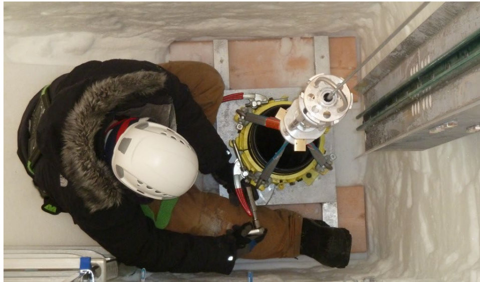
Figure 43: Loosening the toggle clamp U-bolt nuts with a socket wrench to remove the upper casing clamp.
