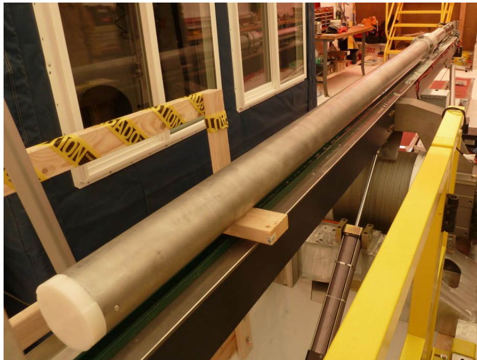
Figure 41: Reamer assembly sitting on the drill tower. Note: this photo is of the reamer in use with the Foro 1650 system.
