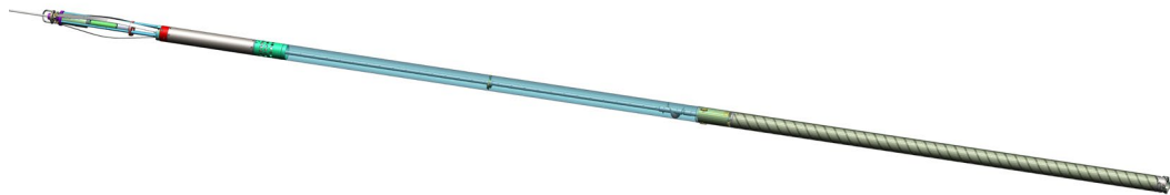
Figure 32. Foro 3000 sonde assembly. The chip chamber and core barrel outer tube are shown transparent to show the internal components.
