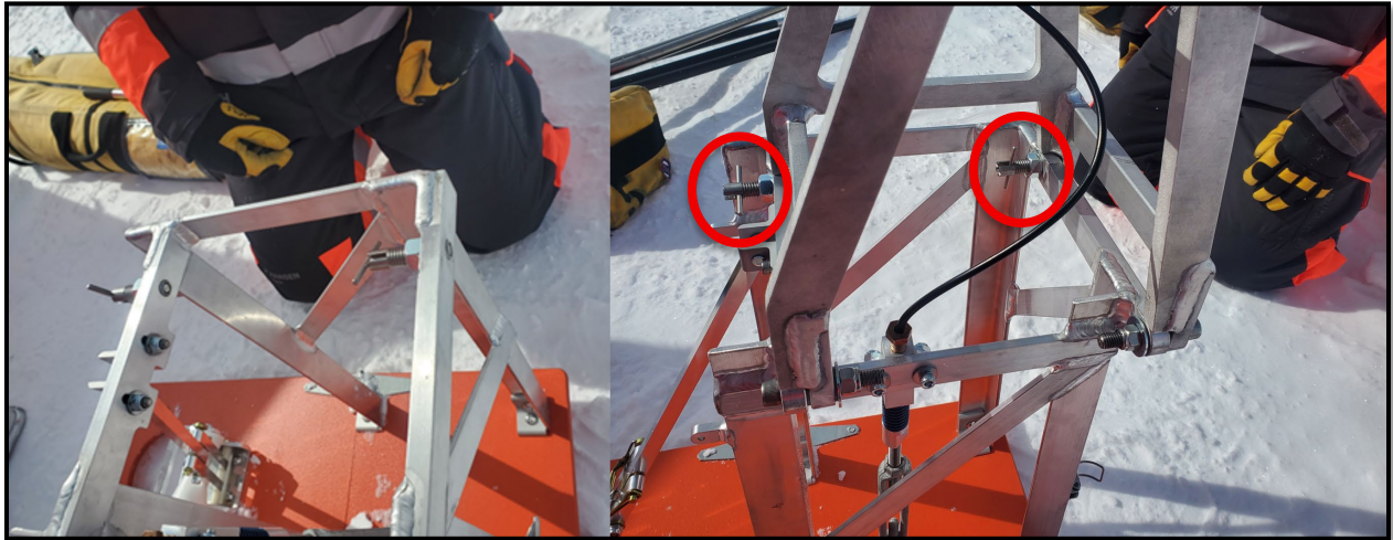
Figure 6: Hinge the upper tower section into place and secure in place with the t-handle detent pins.
