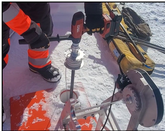
Figure 10: Sidewinder Drill connected to the end of the drill string for coring operations.
