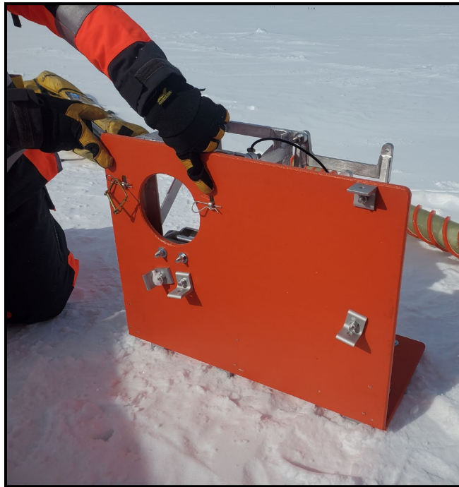
Figure 4: Remove two large cotter pins to unfold the tower platform.
