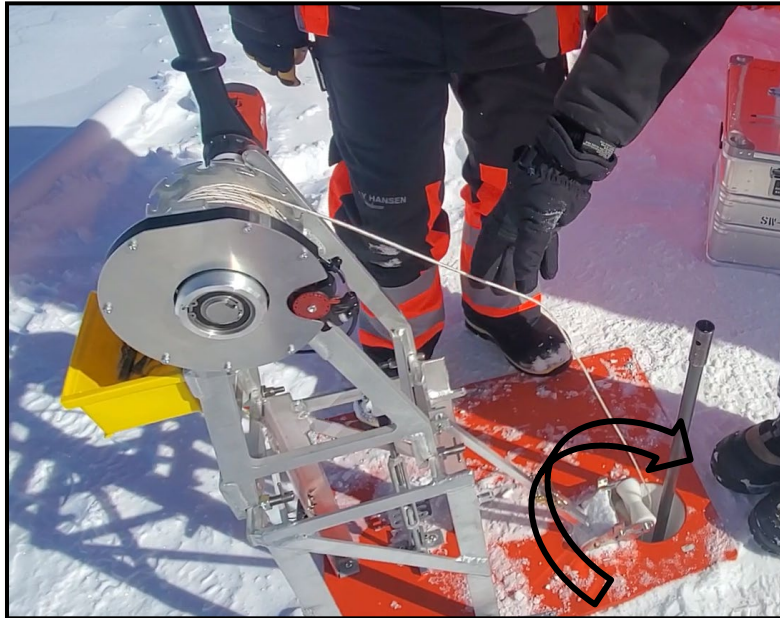
Figure 13: Verify the Sidewinder rope is properly routed, and the pulley is flipped down as shown above before lifting the drill string.
