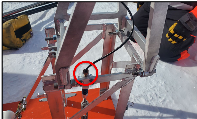
Figure 17: Brake adjustment screw circled in red.
