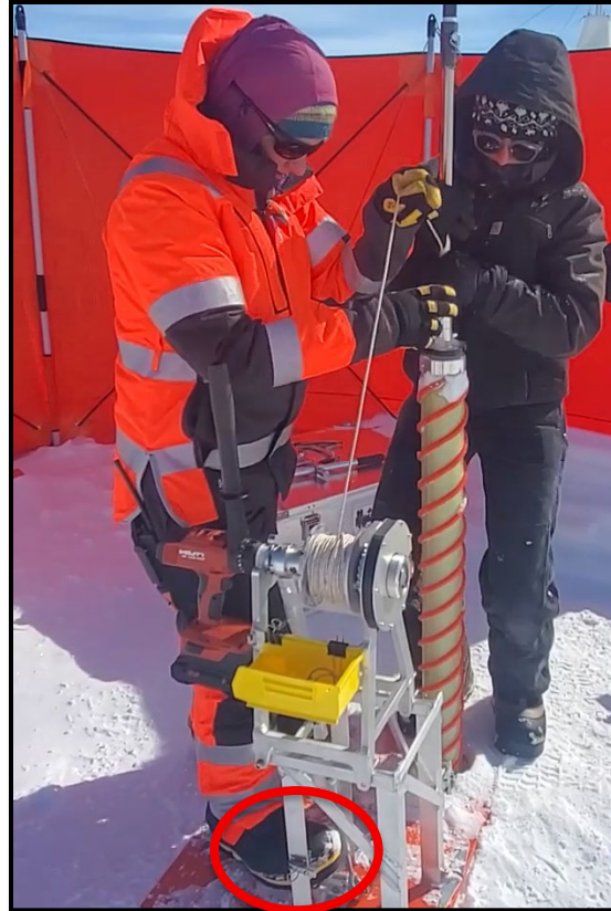
Figure 14: Lifting the core barrel out of the borehole. Operator should disengage the collar and step on the brake release pedal (circled in red) to pay out spare rope to ease extraction of the core barrel.
