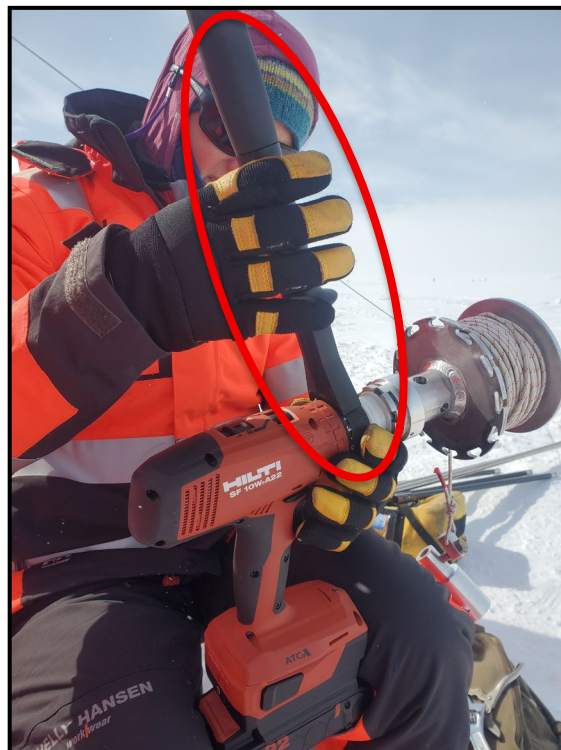
Figure 3: Installing the Sidewinder handle circled in red.
