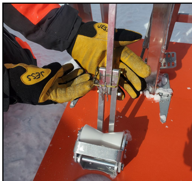
Figure 5: Install the golden clevis pin through all three tower struts to lock the platform in place.
