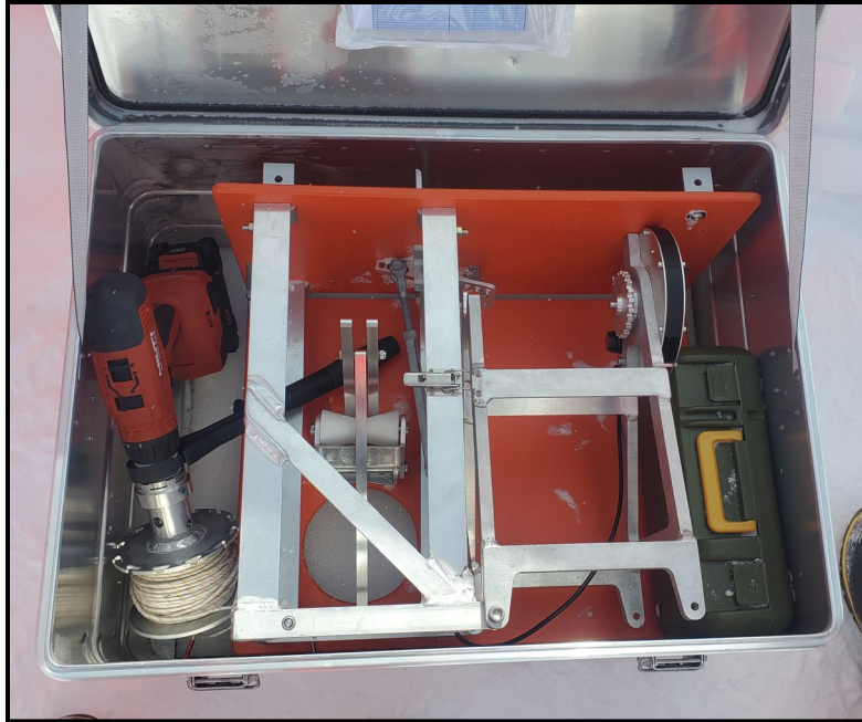
Figure 2: Sidewinder kit as packed for shipping. Sidewinder drill pictured on the left next to the tower assembly on the right.
