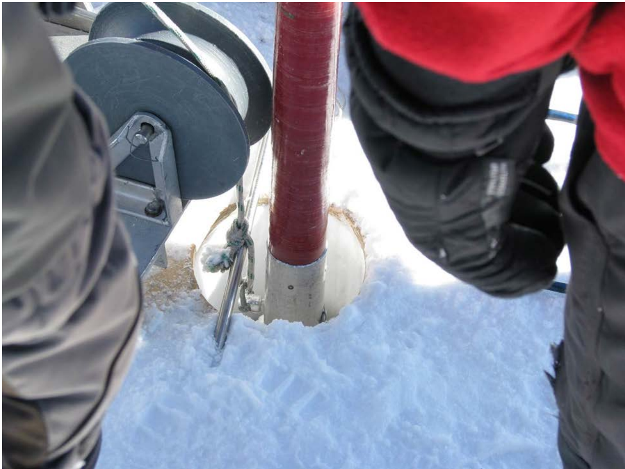
Figure 6: Engaging or disengaging the winder means that the weight of the drill string will need to be transferred to the big \frac{1}{2} -inch rod. The \frac{1}{2} -inch diameter screwdriver shaft, or a \frac{1}{2} -inch rod, is inserted through the loop where the rope is attached to the rope pin. This relieves the rope tension so that: 1) Excess rope can be spooled out to have enough slack to lift the barrel from the hole when coming out of the borehole; or, 2) excess rope can be spooled up so that the rod can be removed--then the winder is ready to lower the drill string when going back into the hole.
