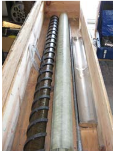
Figure 2 – Prairie Dog inner and outer barrels with core trays
