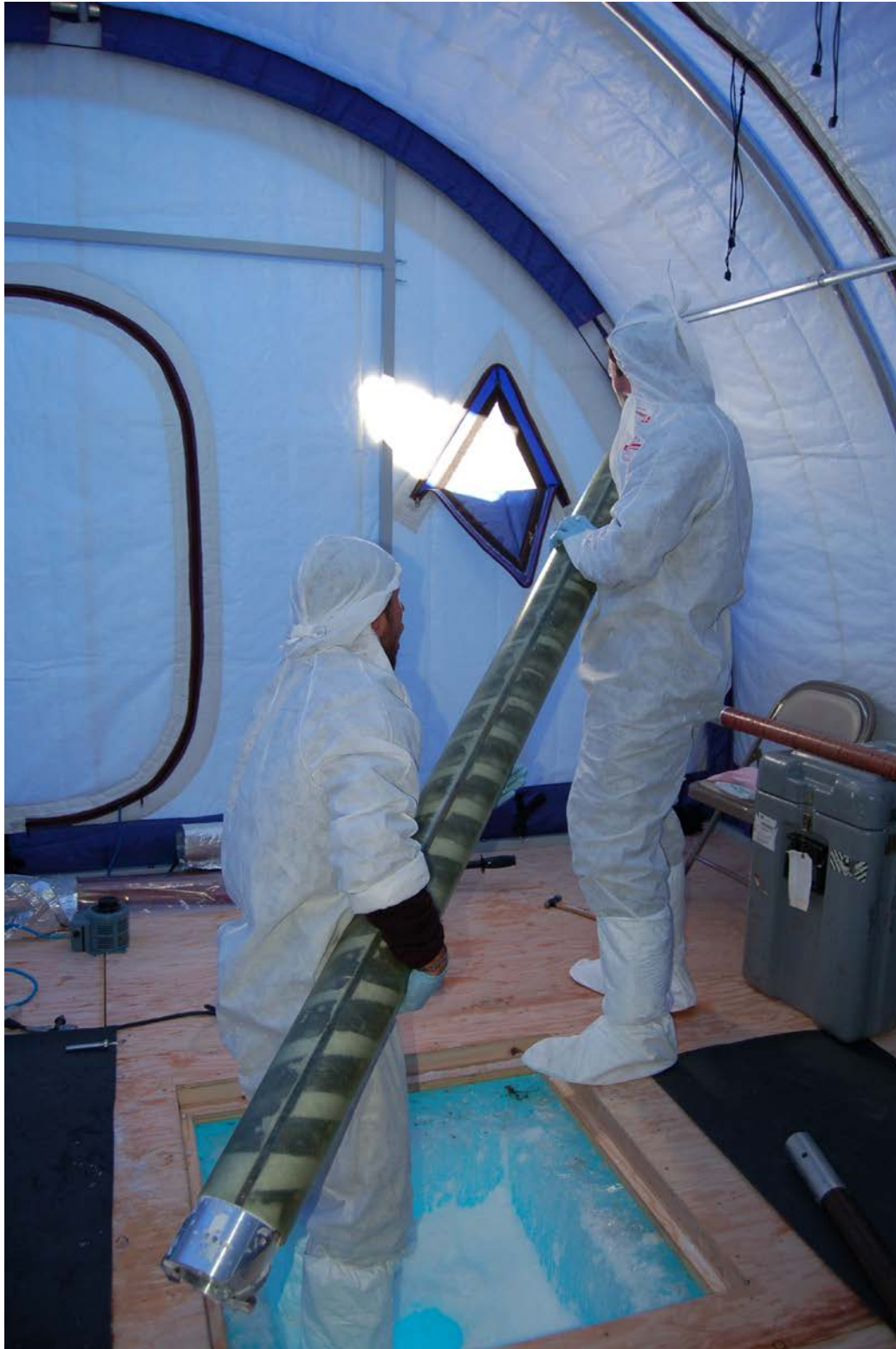
Figure 1 - The Prairie Dog being removed from a borehole. Through the semi-transparent outer barrel ice chips can be seen resting on the flights of the inner barrel.
