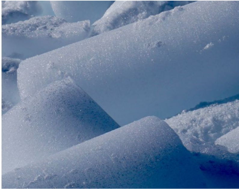
Figure 32. Grooving on the surface of firn cores.
