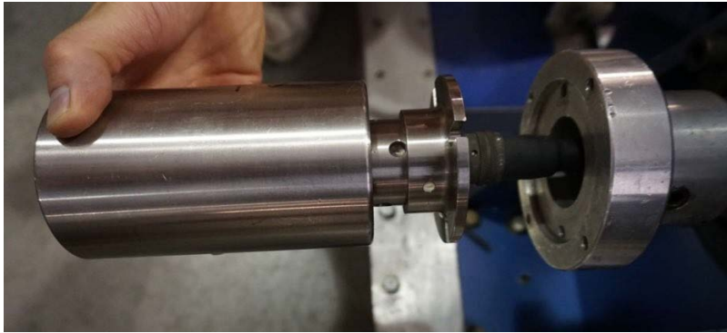
Figure 7. Mounting the slip ring on the winch shaft.
