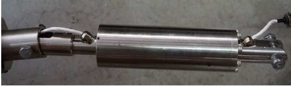
Figure 10. Motor section slip ring attached to the top of the anti-torque.
