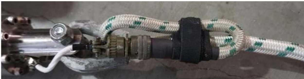
Figure 11. Winch cable connected to the motor section slip ring. Cable pigtail is coiled and secured with a hook and loop strap.
