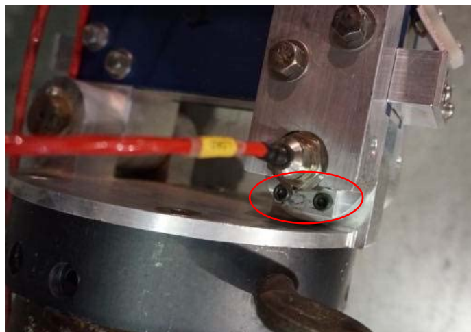
Figure 23. Load cell mounted in the sheave assembly. The keeper plate is circled in red.
