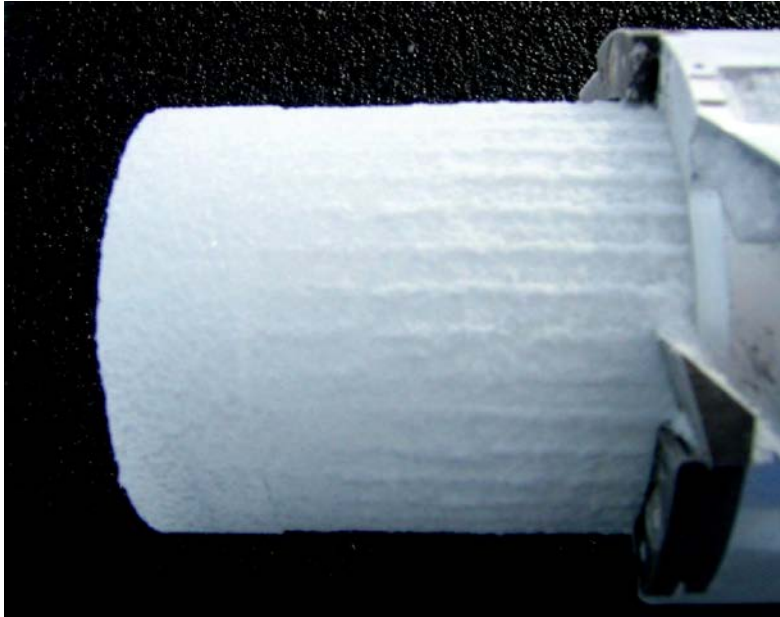
Figure 34. Collet sliding on the surface of the core before break.
