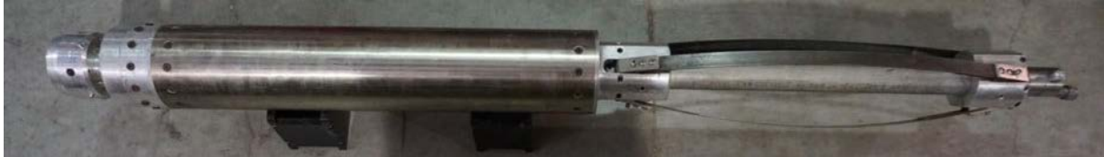
Figure 8. Motor section with anti-torque.
