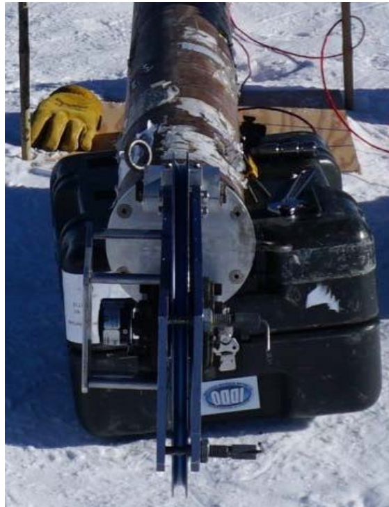
Figure 22. Cable payout encoder under protective plate.
