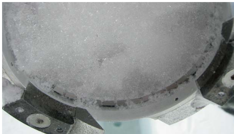
Figure 33. Proper collet core break.
