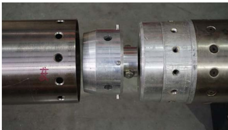
Figure 9. Motor section to outer barrel connection.
