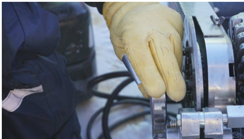
Figure 31. Controlling dill penetration rate with hand wheel.
