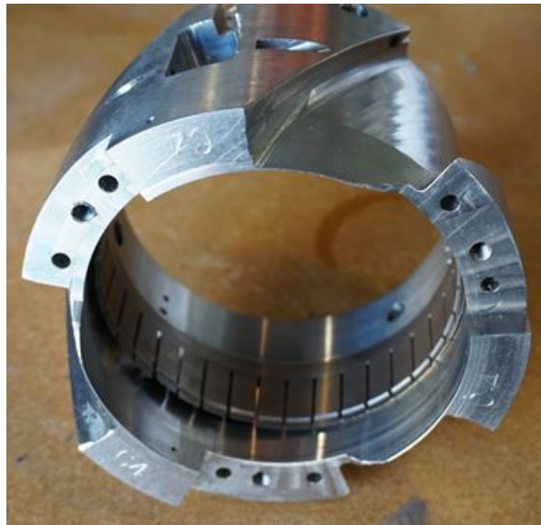
Figure 14. Cutter head with collet-type core catcher.
