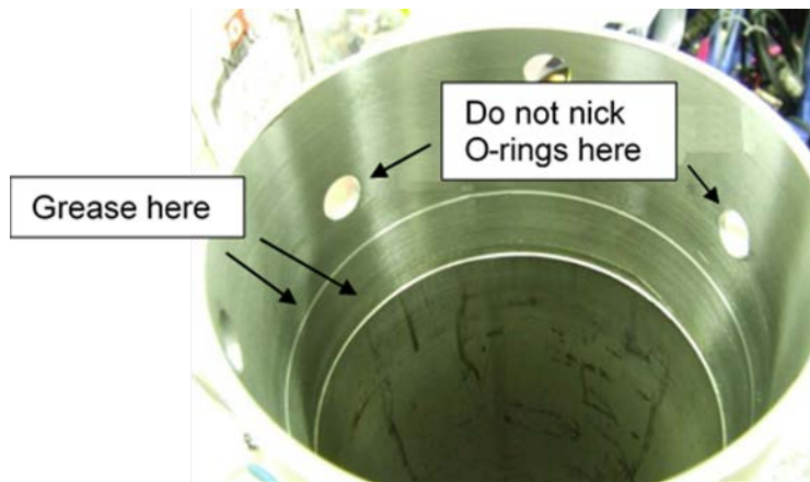
Figure 48. Installing Pressure Sealing O-rings
