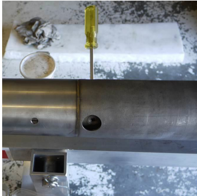
Figure 36. Engaging the Corelocks
