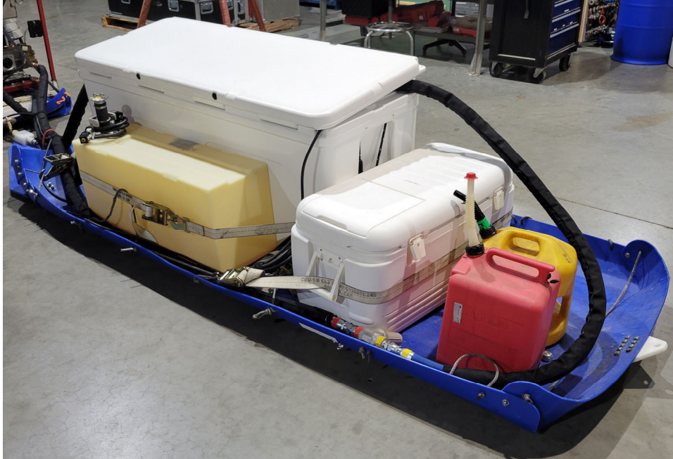
Figure 10: Yeti water tank, fuel tank, and glycol tank secured to the Siglin sled using the supplied ratchet straps.
