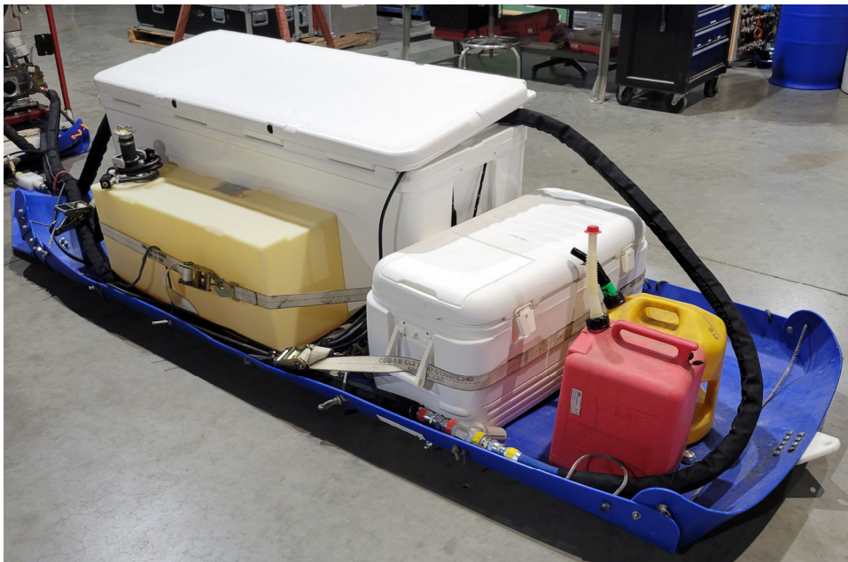
Figure 3: Sled containing the water tank (large white tank), fuel tank (yellow color tank), and glycol tank (small white cooler/tank).
