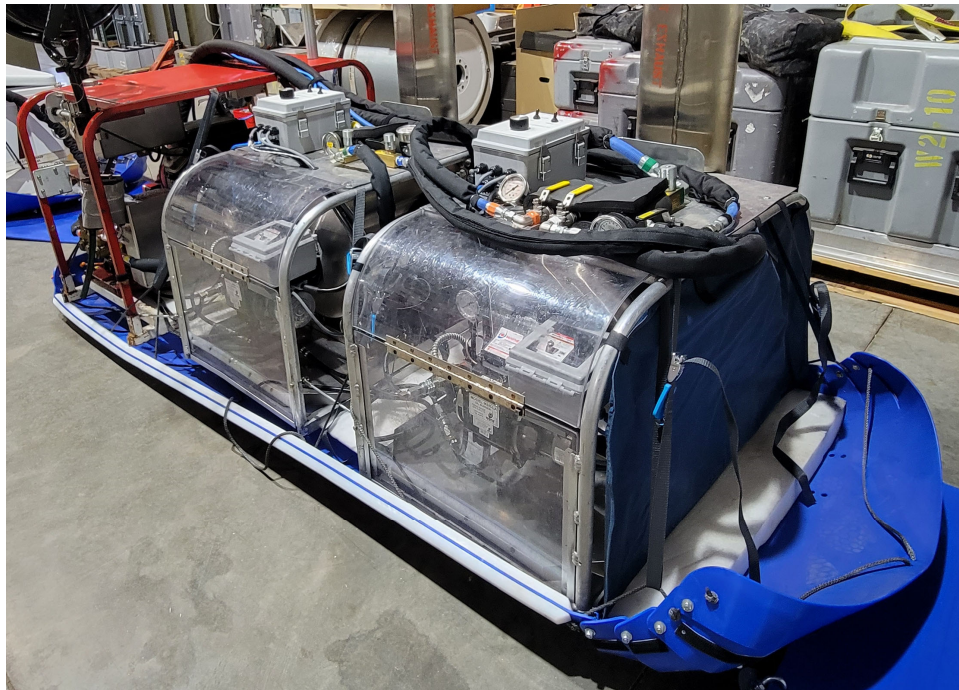
Figure 9: Engine and heater modules secured to the Siglin sled using the supplied cam straps.
