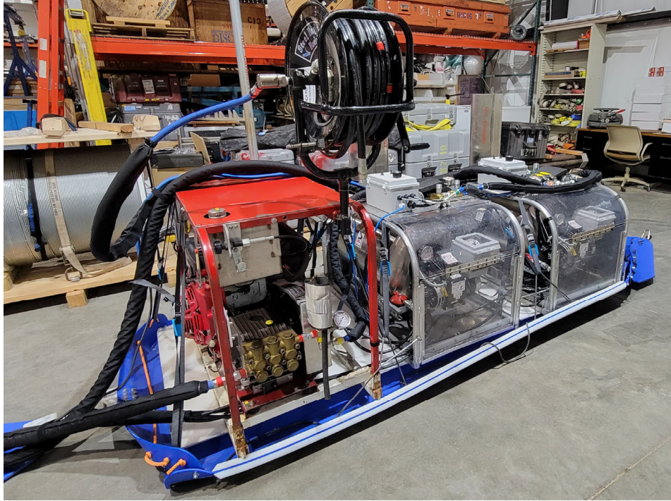
Figure 2: Sled containing the pump/generator (red unit) and heaters (two silver-colored units).
