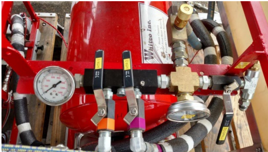
Figure 6: Hot manifold above Heater 2. Hot water in from heaters in middle with shutoff ball valves, bypass to tank with main flow control valve heading out back, and drill supply with valve and vacuum break on right side.
