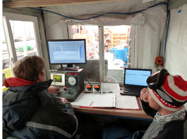
Figure 16. Drill control interface inside the control room tent.
