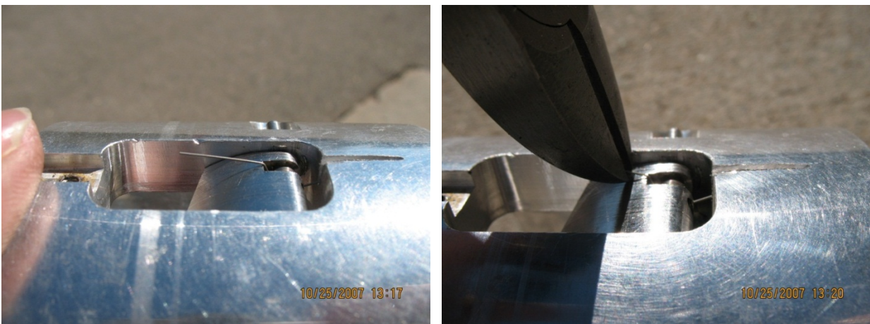
Figure 10: Core Dog Spring Bend and Trimming
