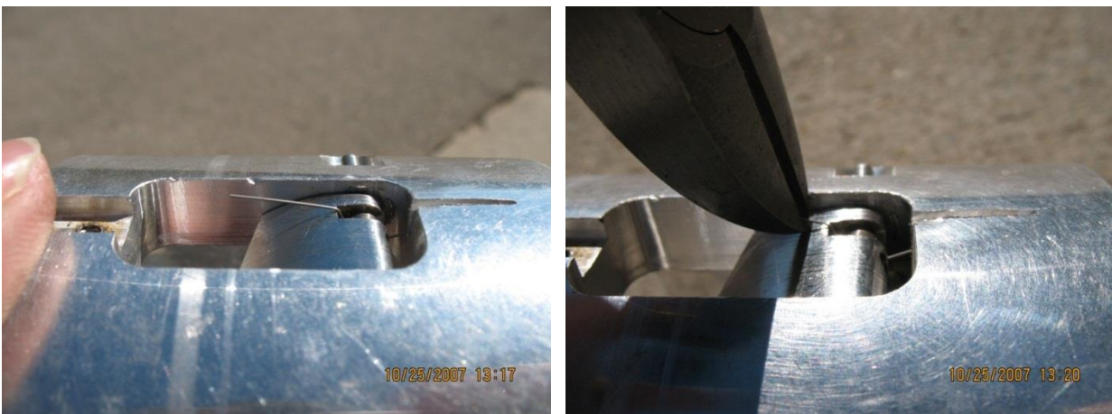
Figure 10: Core Dog Spring Bend and Trimming
