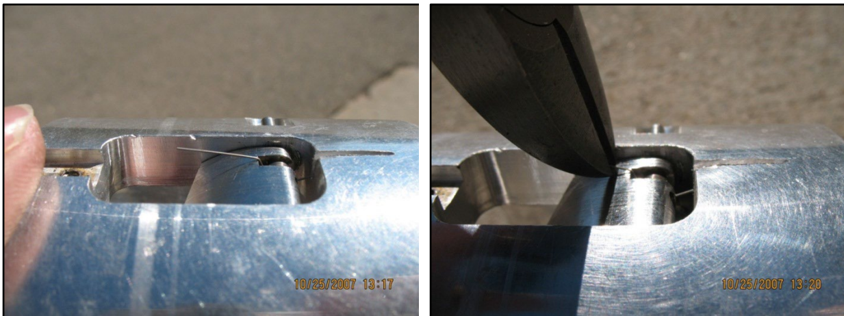
Figure 11: Core Dog Spring Bend and Trimming
