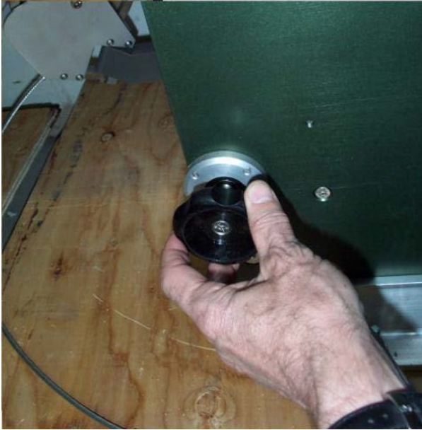
Figure 7: Level-wind adjustment knob
