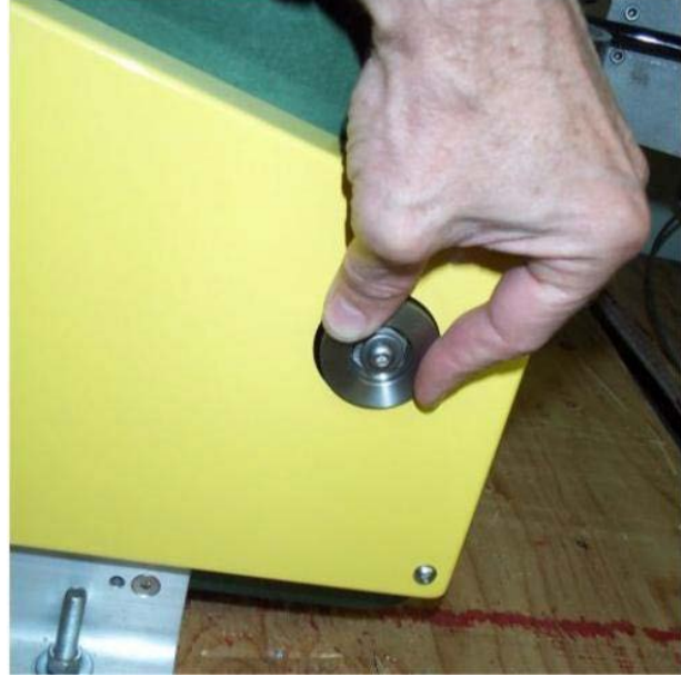
Figure 8: Level-wind clutch button
