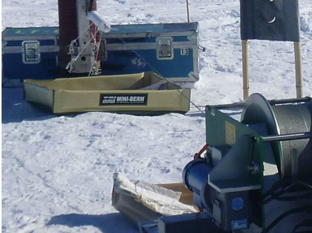
Figure 3: Simple cable wipe setup
