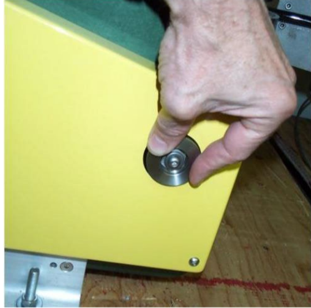
Figure 8: Level-wind clutch button
