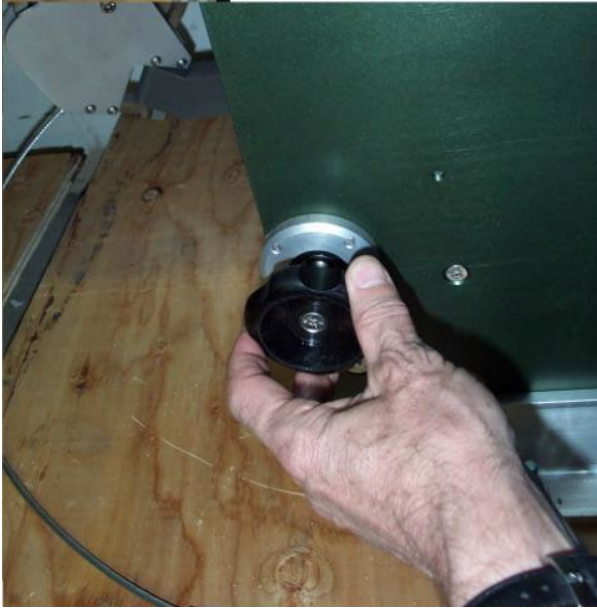
Figure 7: Level-wind adjustment knob
