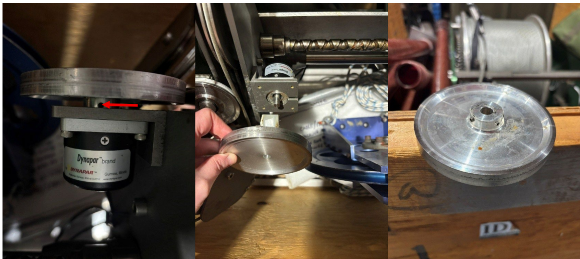
Figure G.3: Aluminum wheel removal.
