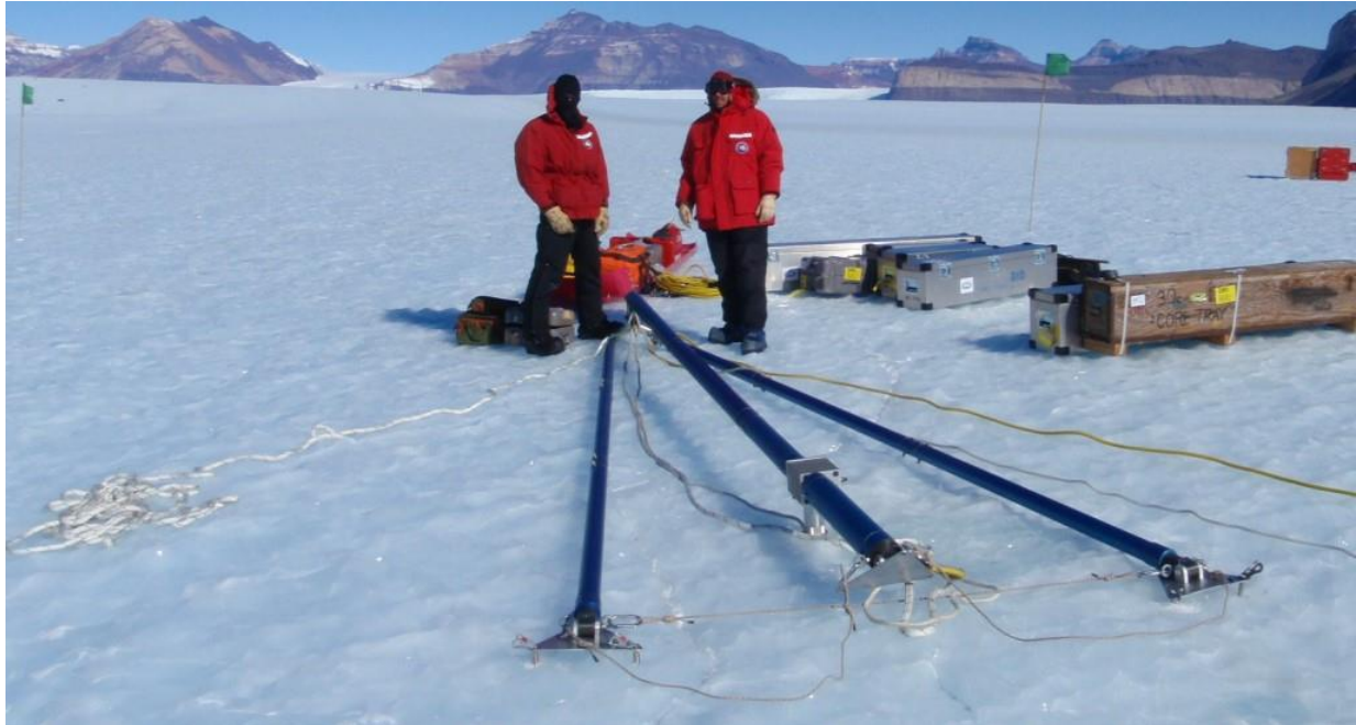
Figure 2: BID Tripod ready for standing. Note the position of the Footplates, ice screw anchors, and Safety Ropes between legs. Ropes and Electrical Cord have been installed and laid-out so as to not interfere with Tripod standing.
