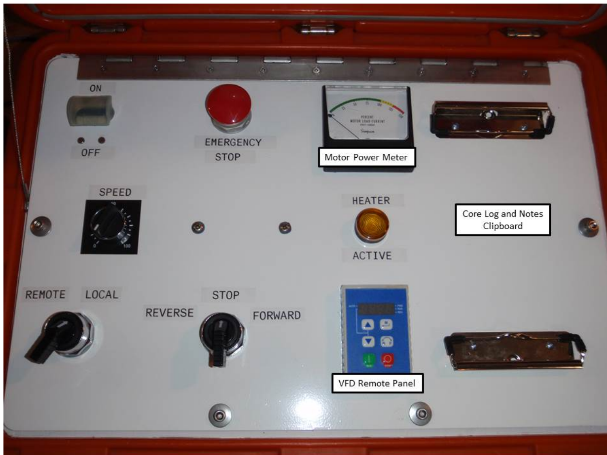
Figure 7: BID Control Box Faceplate.
