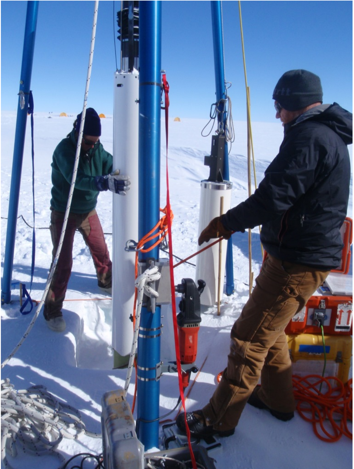
Figure 16: Removing the Core Barrel after a coring run with the Motor Section with Anti-Torque Assembly.
