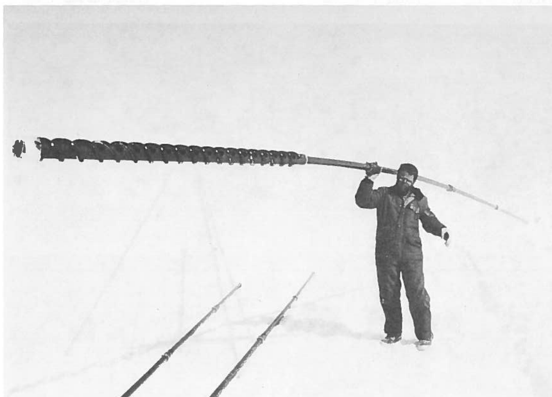
Figure 2. PICO driller with 9 m of extensions.
