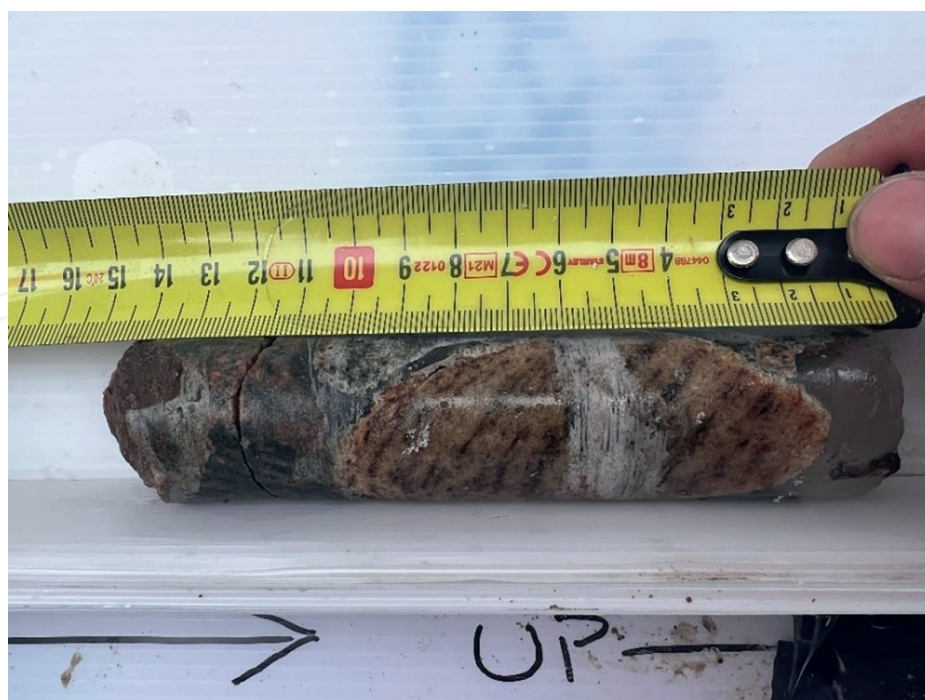
Figure 11. Core from the ice-enabled Winkie drilling near Prudhoe dome (photo credit: Jason Briner).
