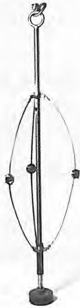
Figure 11. Temperature probe mount.
