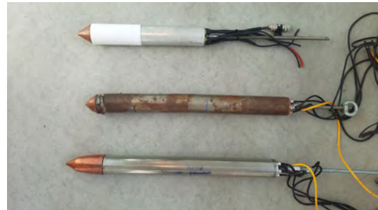
Figure 3. Photograph of the v1 (top), v2 (middle), and v3 (bottom) melt-tip versions developed over the 3-year project lifetime (v0 not shown). The v2 melt tip shown here, which has been sectioned for destructive testing, bears a characteristic rust coating that develops with melt-tip use. The v1 and v3 melt tips shown here have not been used.
