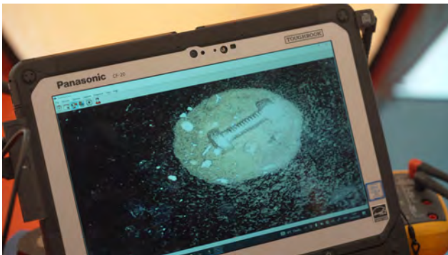
Figure 22. A down-borehole video camera shows substantial sediment accumulation on the borehole bottom within 5 m of the ice surface. We estimate that a water-filled cavern of diameter \sim 50 cm formed around the melt tip. A bolt of length \sim 1.5 cm was dropped into the frame for scale.
