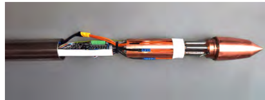
Figure 5. Overview of the internal construction of the melt tip before resin casting.
