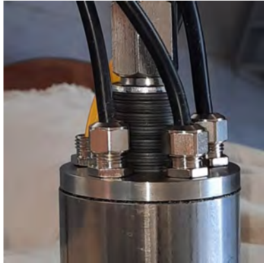
Figure 7. With four power cables, one data cable, and an M10 threaded bolt covered in Belleville washers, there is very little free space on the metal top cap of the lower member of the melt tip.
