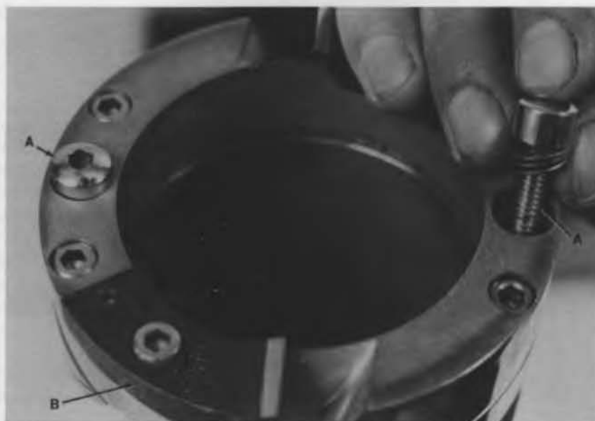
Figure 4. Cutting shoe for SIPRE/CRREL auger, showing elevating screws (a) and replaceable cutters (b).
