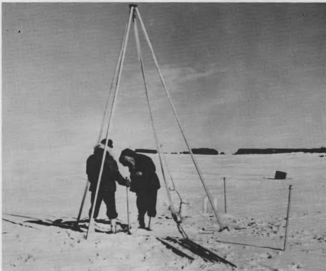
Figure 10. Deep coring with the aid of a light tripod for lifting and lowering.
