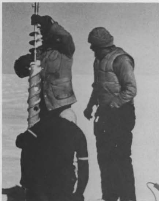
Figure 18. Rand drill with section of flight auger for stirring cuttings above the core barrel.
