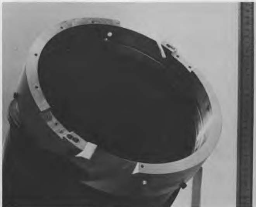
Figure 23. Cutting head of 12-inch auger (one cutter and both elevating plates have been removed in this photo).
