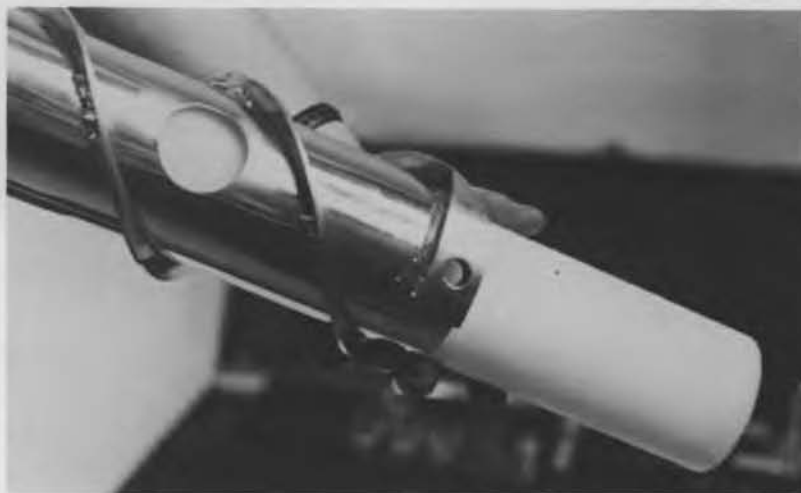
Figure 5. Core being removed from the upper end of the core barrel of the 3-inch auger (driving head removed).
