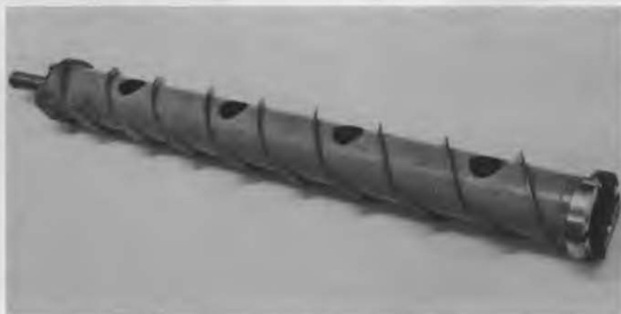
Figure 2. The 1-m-long core barrel of the SIPRE/CRREL 3-inch ice auger.
