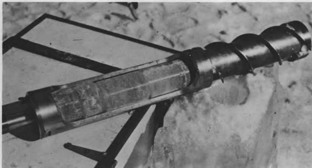
Figure 1. The original ACFEL ice coring auger, showing the core barrel and the attachment for removing cores.
