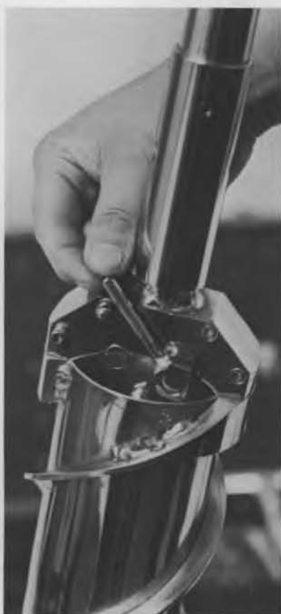
Figure 6. Driving head on the 3-inch SIPRE/CRREL auger.
