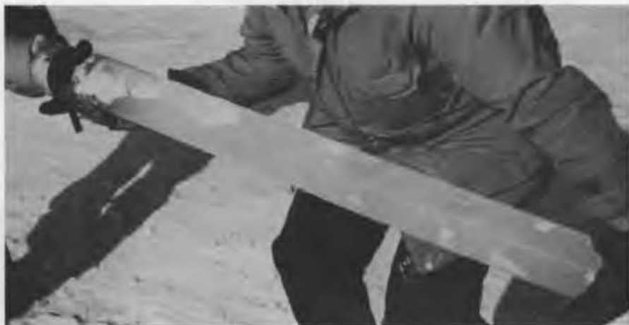
Figure 20. Core of multi-year sea ice produced by the prototype Rand auger.
