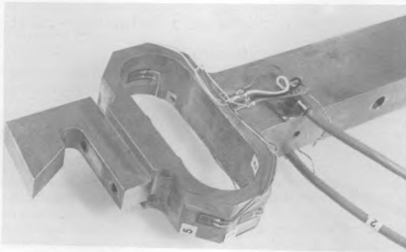
Figure 2. Force dynamometer and cutter assembly.
