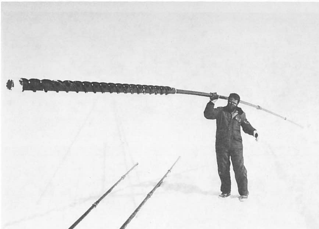
Figure 2. PICO driller with 9 m of extensions.
