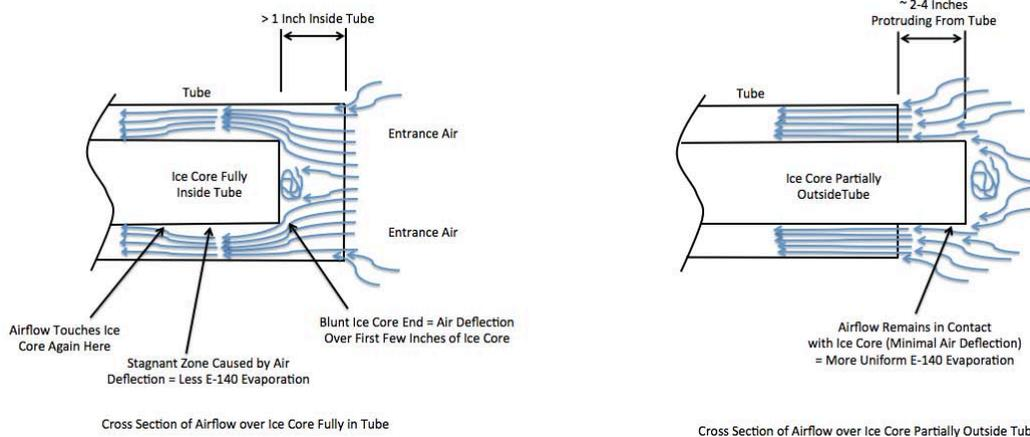
**Figure 27 – E-140 Evaporation Uniformity Improvement with Ice Core Protrusion**
