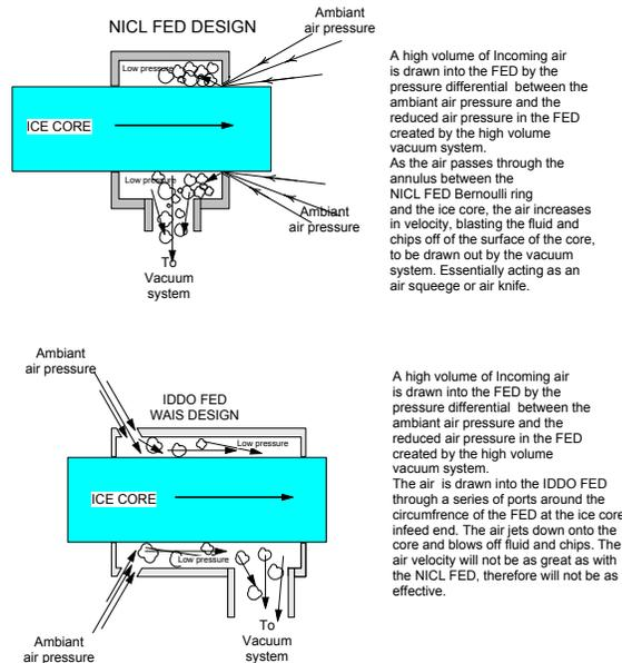
**Figure 20 - Differences between the NICL FED and the IDDO FED**
