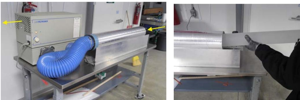
Figure 22 – Ad Hoc Feasibility Test at NICL (GAC Filter is Inside Blower Housing)
