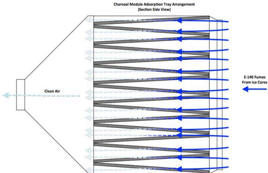
**Figure 13 - Accordion-Like Charcoal Tray Arrangement In Charcoal Module
