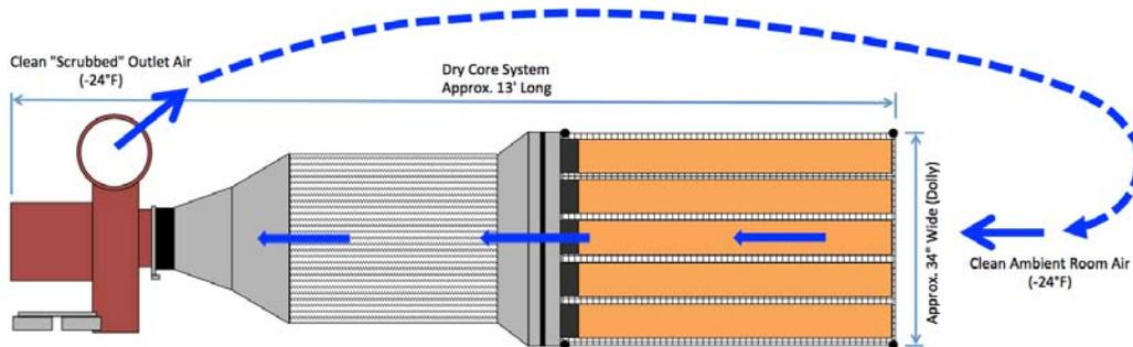
**Figure 17 - Top View of Connected Dry Core Modules**
