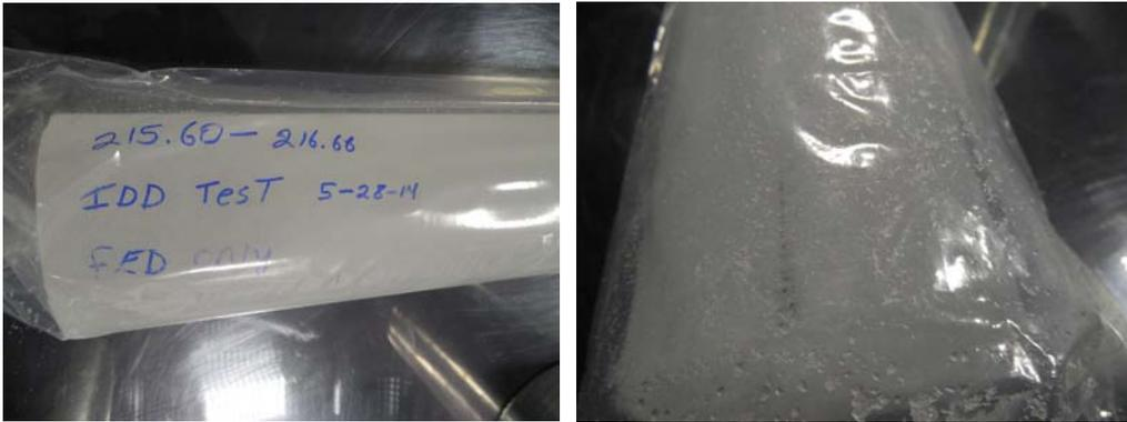
**Figure 2 – Estisol-140 Residue on Example of Greenland Ice Core and Storage Bag**
