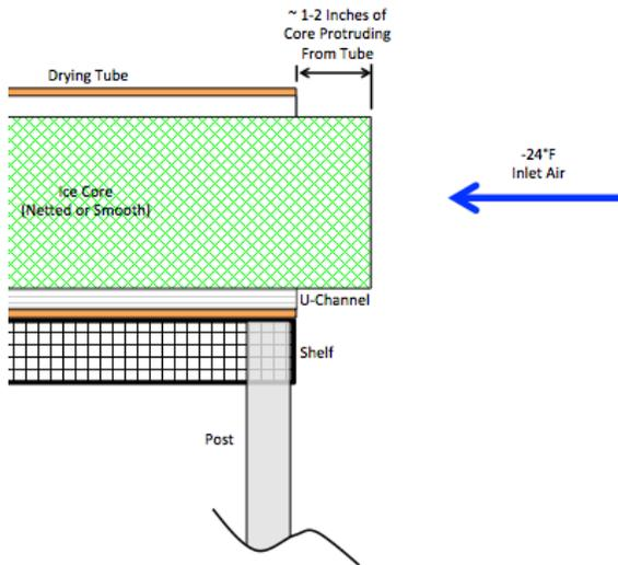
Figure 11 - Entrance End of Drying Tube
