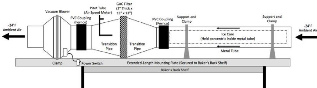
Figure 24 - Conceptual Layout (One Blower and GAC Filter per Ice Core)
