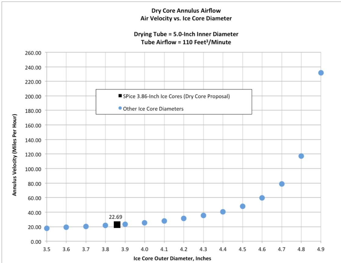
**Figure 31 - Velocity Increases Dramatically with Various Core Diameters in 5-Inch Drying Tube. (Note: A 4.1-Inch Core Diameter is the Suggested Maximum in a 5-Inch Tube Due to Increasing Air Speed (i.e., Air Friction and Pressure Drop))**
