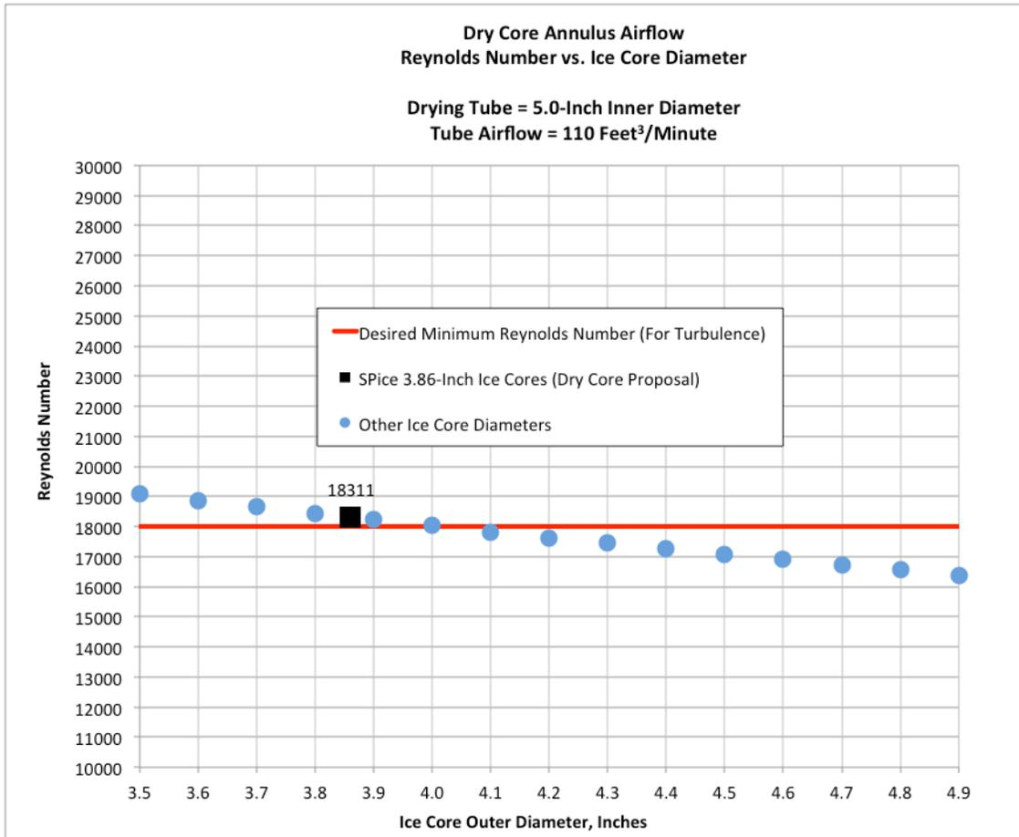
**Figure 30 - Reynolds Number is Relatively Stable with Various Core Diameters in 5-Inch Drying Tube**
