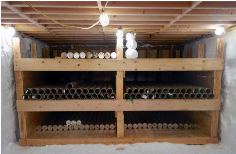
**Figure 5 - South Pole Brittle-Ice Cores "Relaxing" at South Pole Drill Site**
