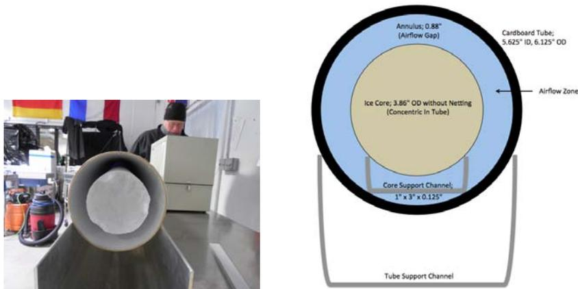
Figure 23 - Ice Core Concentric In Tube for Feasibility Test
