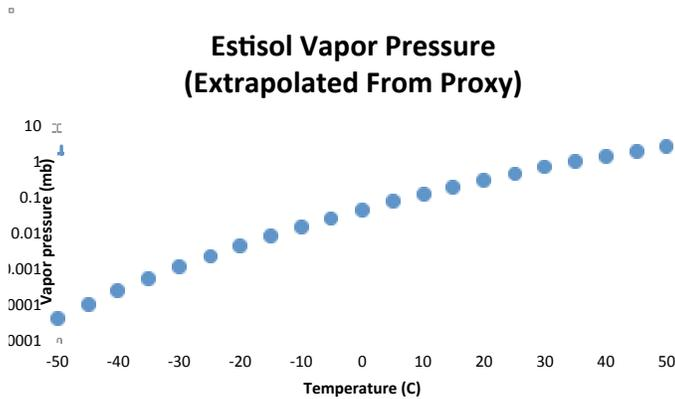
**Figure 25 - Estimated Vapor Pressure for Estisol-140 Based on a Similar Compound**
