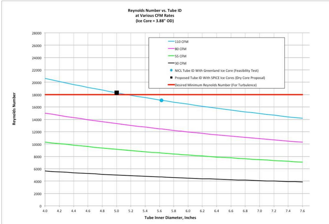
**Figure 29 - Reynolds Number With Varying Airflow Rates and Tube Diameters**
