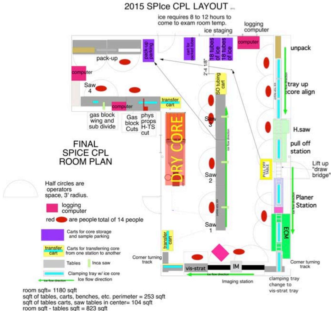
**Figure 6 - NICL Exam Room Layout Ice Core Processing for SPice Ice Cores, with Dry Core System Shown for Scale (Plan View)**
