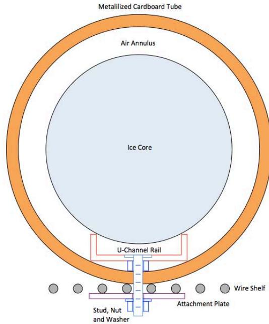
Figure 9 - Cross Section of Typical Ice Core Located Concentric In A Drying Tube
