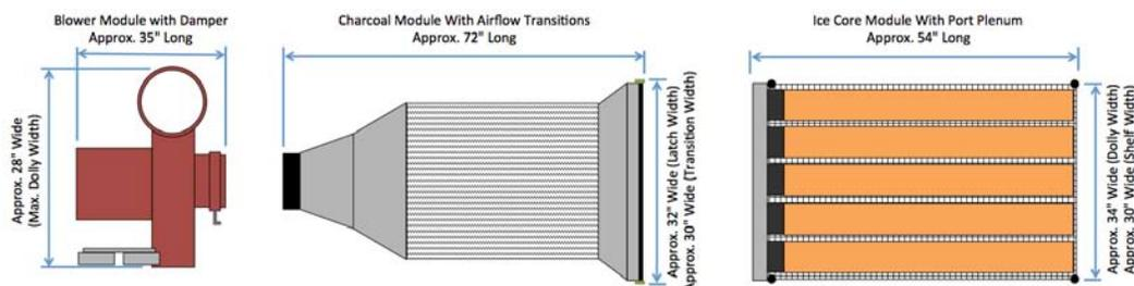
Figure 16 - Top View of Separated Dry Core Modules
