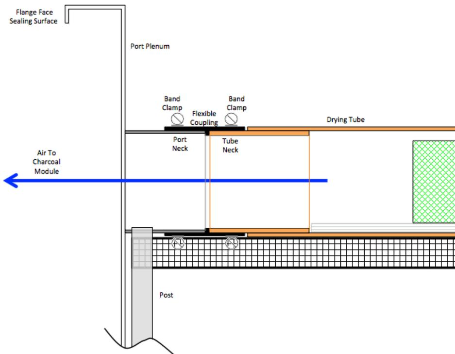
Figure 12 - Exit End of Drying Tube
