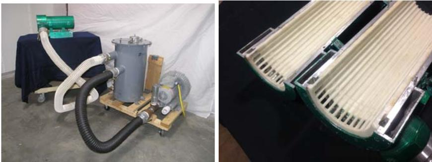
**Figure 19 - Fluid Extraction Device (FED) System, and Detail of the NICL FED Air-Knife**
