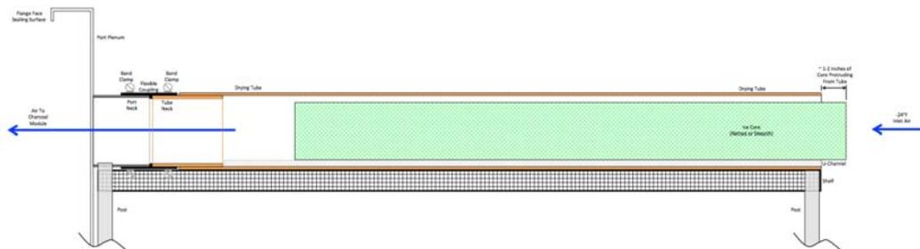
Figure 10 - Section Side-View of Ice Core In Drying Tube On A Shelf, Connected To Port
