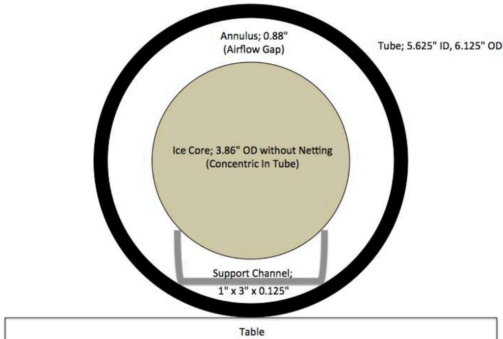
**Figure 28 - Ice Core In Tube as Tested at NICL**
