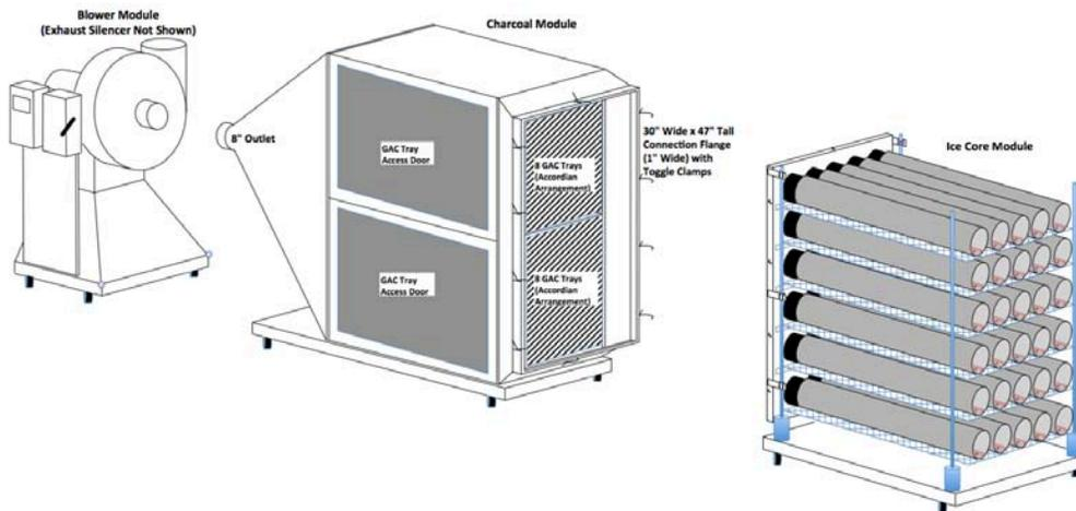
Figure 7 - Separated Dry Core Modules
