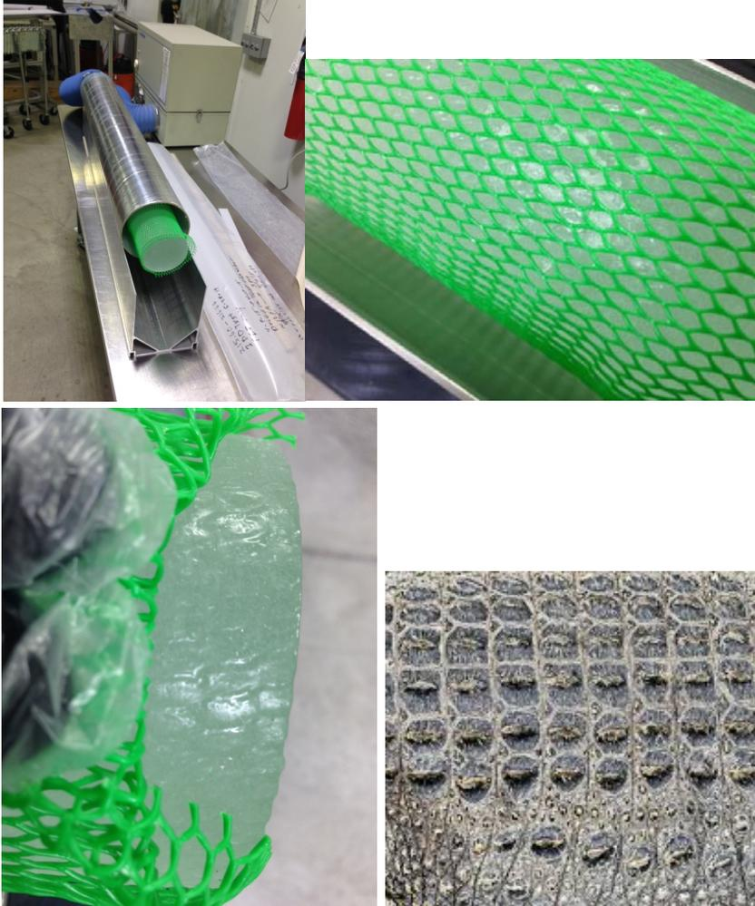
**Figure 26 - Netted Core with “Alligatoring” of Ice Surface (Differential Sublimation), and a Photo of Alligator Skin**
