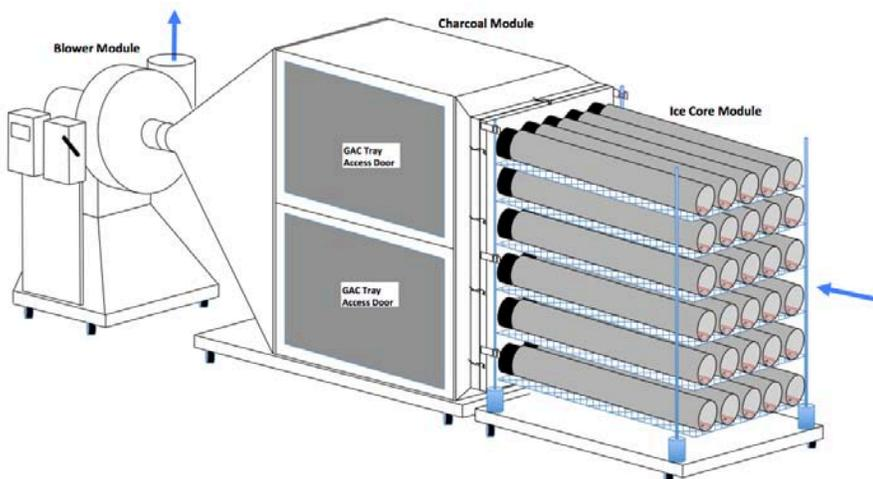
Figure 8 - Connected Dry Core Modules
