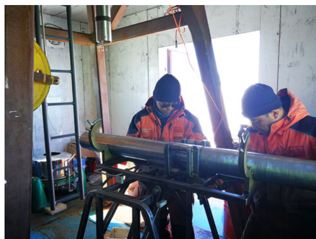
Fig. 11. Screwing/unscrewing trolley in operation at the Zhongshan Station, Antarctica.
