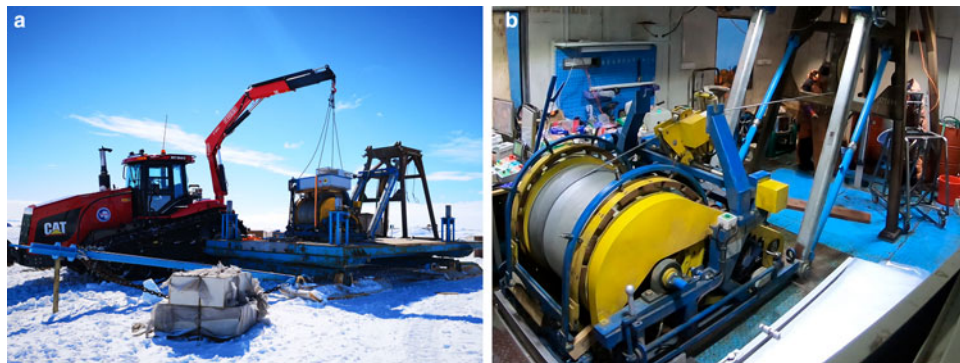
Fig. 5. Drilling winch system: (a) unloading into the movable drilling shelter at Zhongshan Station, Antarctica and (b) view of the drilling winch inside the shelter.
