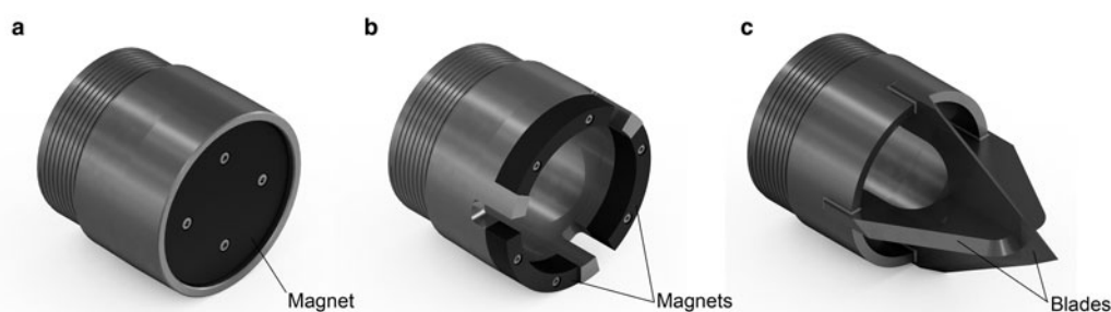
Fig. 15. Fishing tools: (a) full-diameter magnetic drill head, (b) annular magnetic drill head and (c) conical drill head.
