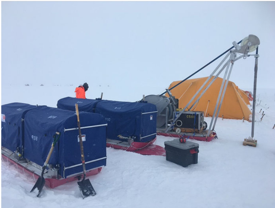
Fig. 2. The RAM-2 Drill system includes improvements to all major sub-systems. Visible from right to left are two sleds with four air compressors under blue covers and the hose reel sled with hose, control box, generator in black case, tower and sonde.
