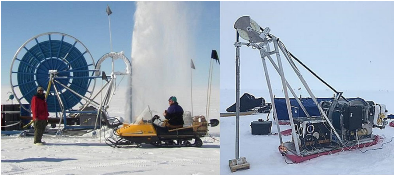
Fig. 4. The original RAM hose reel and tower 5.6 m × 2.4 m × 3.7 m (L × W × H), 2800 kg (left) and the reduced-size RAM-2 hose reel and tower 3.7 m × 1.1 m × 2.8 m (L × W × H), 560 kg (right).
