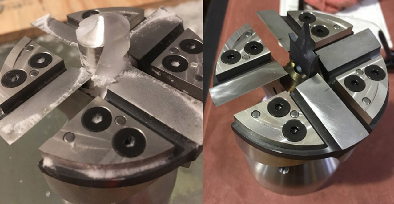
Fig. 8. The RAM-2 cutter head was modified to address clogging seen on the original twist bit (left). Improved chip clearing was seen using the spade cutter (right).
