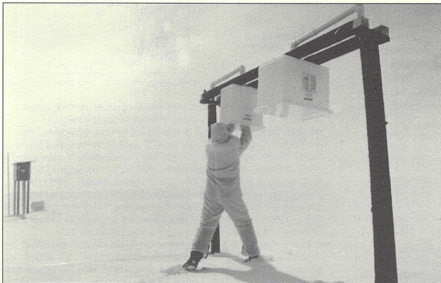
At the atmospheric sampling site (ATM) great effort is taken to sample air that has not been affected by the GISP2 camp or other sources of local contamination. This site may be the "cleanest" atmospheric sampling station in the world. Here a researcher changes a filter. The aerosols in the air, trapped on this filter, will be analyzed for their trace metal content. (Photo: Jack Dibb)
