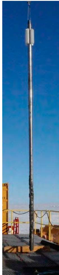
Figure 20. WISSARD/Caltech piston corer with sediments packed at lower part [8] (Reproduced with permission from Royal Society, 2016).
