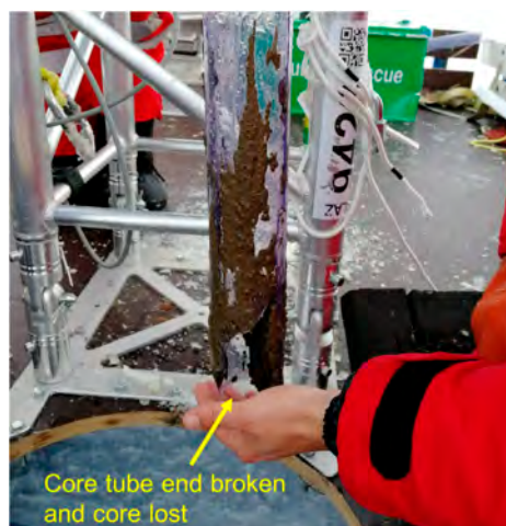
Figure 30. Broken tube end of gravity corer after meeting with hard material in sediments (photograph was taken by Y. Li).
